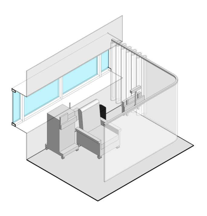
Sheet Description: TYPICAL RENAL DIALYSIS TREATMENT STATION ISOMETRIC Scale: Sheet: 3A
