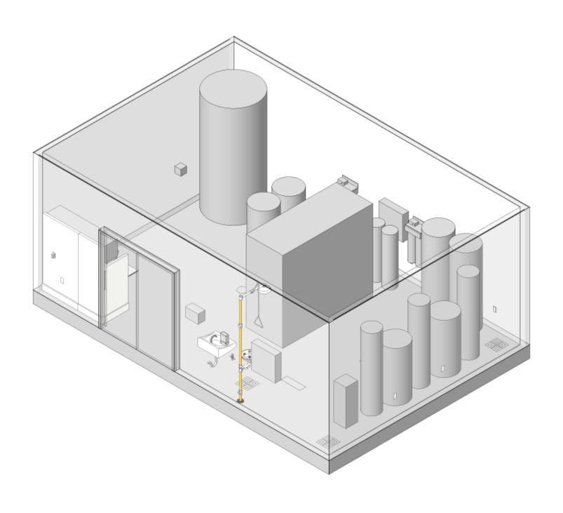
**Sheet** WATER TREATMENT / DILYSATE PREP ROOM ISOMETRIC - 12-28 **Description:** STATION DIALYSIS CENTERS (RCA02)
