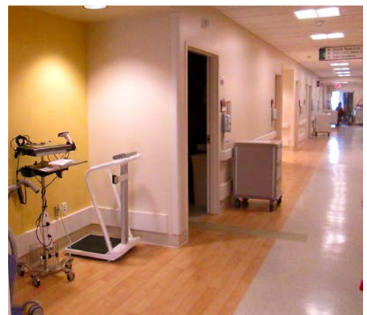
Figure 4.10.7: Niches in hallways allow for supplies to be stored outside of patient rooms, and easily accessed by staff. West Los Angeles VA Medical Center. Los Angeles, California.
