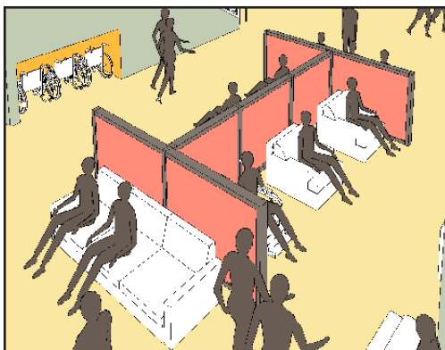
Figure 4.2.3: An example of multiple seating configurations with 54" interior partitions at the back side of seating.
