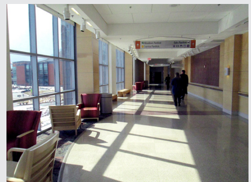
Figure 4.2.17: Single-loaded corridor with generous natural light, casual seating, and display area. Fort Belvoir, Virginia.
