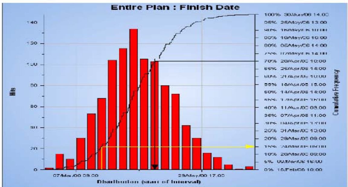
Figure 2. Finish date histogram . The bars on the graph represent how often during the analysis the plan finish on certain date or between a certain date range 1 .
