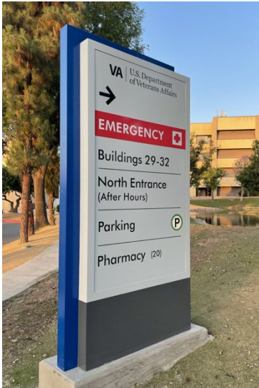
Figure 1-1 (Above) A well-maintained exterior sign system can last 10-15 years. Regular cleaning, paint touchups, electrical maintenance, and message updates will maximize the system's lifecycle.
