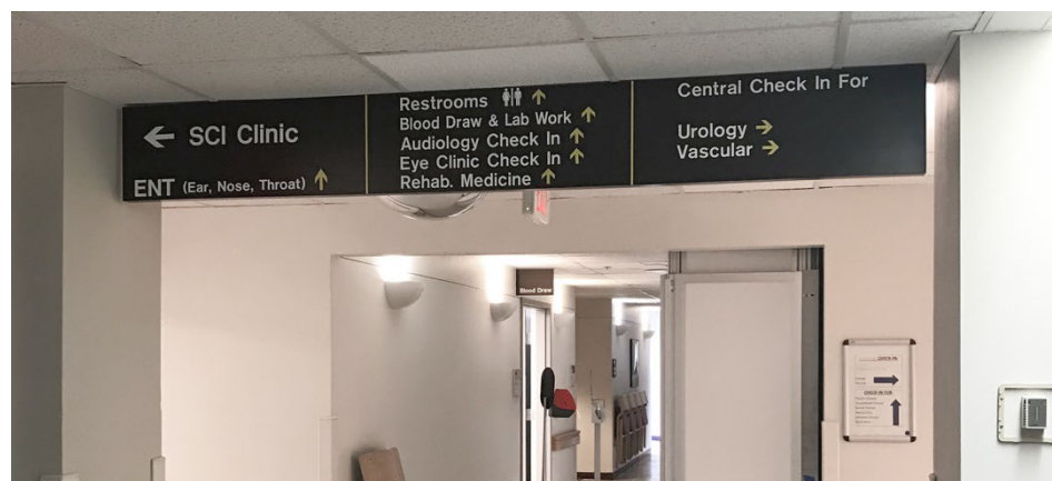
Figure 1-7 (Right) The overhead sign is confusing because it lists too many destinations and the directional arrows are used incorrectly. To minimize confusion, overhead signs should only include a limited number of major destinations. Additionally, a single directional arrow pointing in the direction of travel should be used in combination with wall-mounted signs that provide more detailed information.
