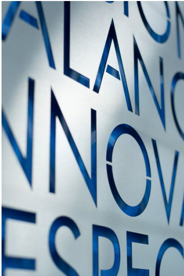
Figure 1-35 Example of text routed from a sheet of brushed stainless steel using a CNC machine
