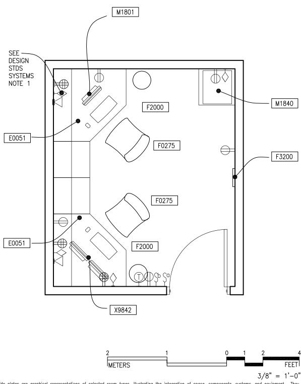
Guide plates are graphical representations of selected room types, illustrating the integration of space, components, systems, and equipment. They provide typical configurations and general technical guidance, and are not intended to be project specific. Specific infrastructure design requirements are contained in VA Design Manuals and Space Planning Criteria located in the VA Technical Information Library.
