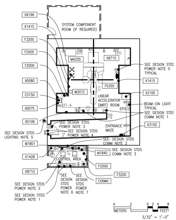
Guide plates are graphical representations of selected room types, illustrating the integration of space, components, systems, and equipment. They provide typical configurations and general technical guidance, and are not intended to be project specific. Specific infrastructure design requirements are contained in VA Design Manuals and Space Planning Criteria located in the VA Technical Information Library.
