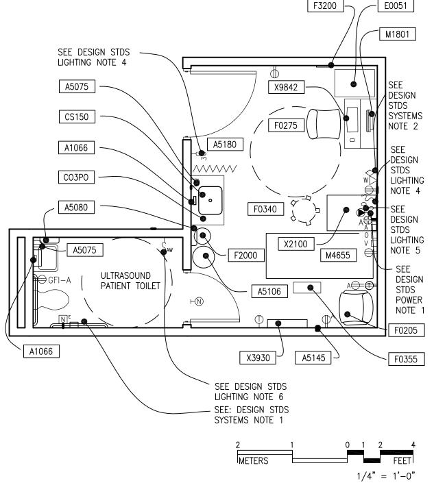
Guide plates are graphical representations of selected room types, illustrating the integration of space, components, systems, and equipment. They provide typical configurations and general technical guidance, and are not intended to be project specific. Specific infrastructure design requirements are contained in VA Design Manuals and Space Planning Criteria located in the VA Technical Information Library.
