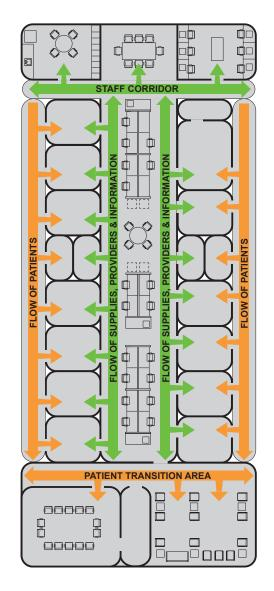
Figure 4.2-5 Three Flows in the Dual Corridor System
