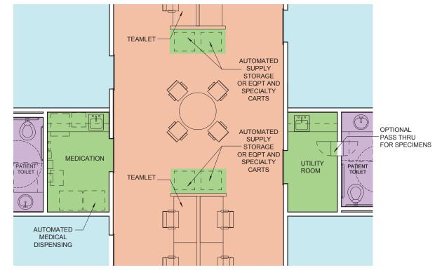
Figure 4.3-27 Enlarged Floor Plan of Core Supplies
