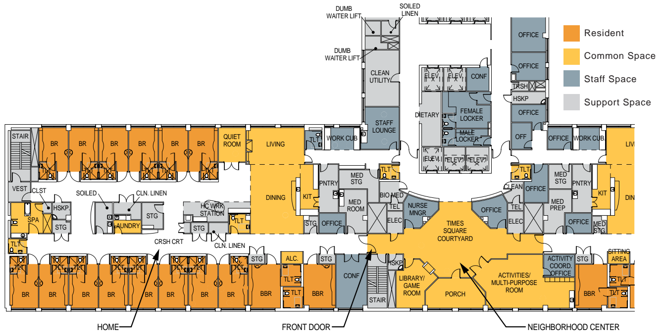
Figure 2.46 Floor plan at Martinsburg VA CLC Renovation.
