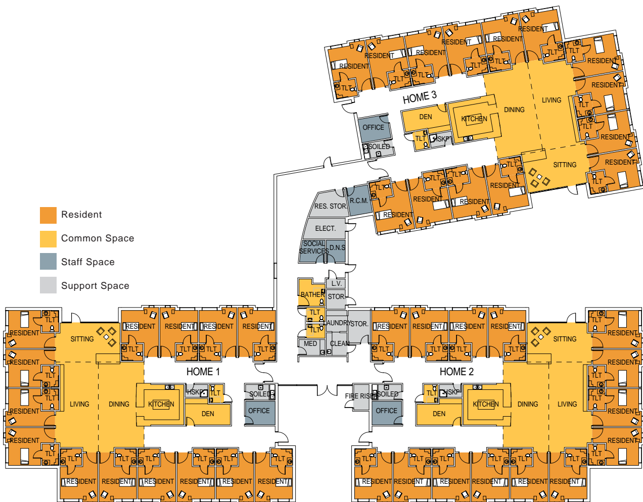
Figure 2.6 The floor plan of Lebanon, OR State Veterans Home exemplifies principles of the Small House Model design, such as locating the kitchen in the center of the house and separating on-stage and off-stage spaces.
