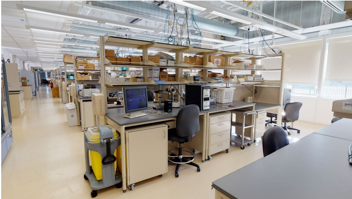
Image A.1 A Lab Bench Unit in the open lab at the Rocky Mountain VAMC R&D Facility includes mobile drawer units and utility drops from the ceiling for adaptability.
