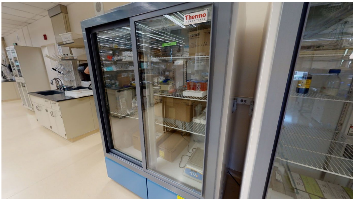
Image A.6 Chromatography cabinets within the open laboratory at the Rocky Mountain VAMC R&D Facility are a cost-effective alternative to cold rooms.
