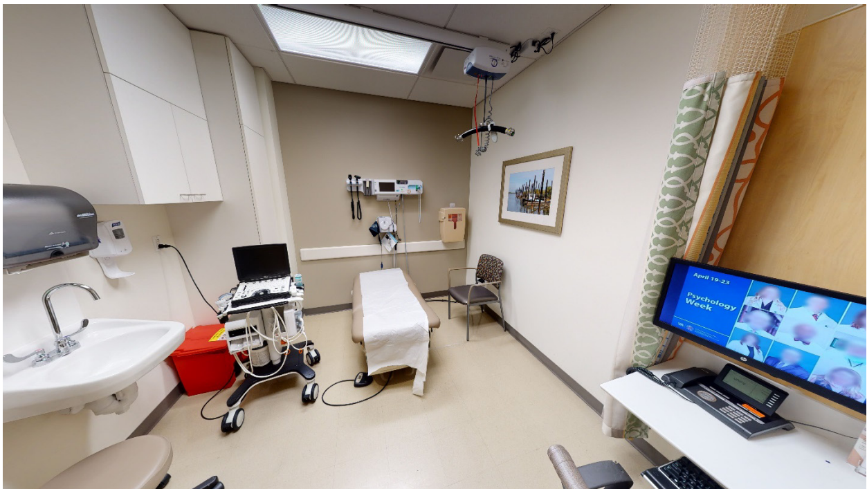
Figure 3.4 The PMR Svc Exam Room tables at the New Orleans VAMC are positioned to provide access on three sides.
