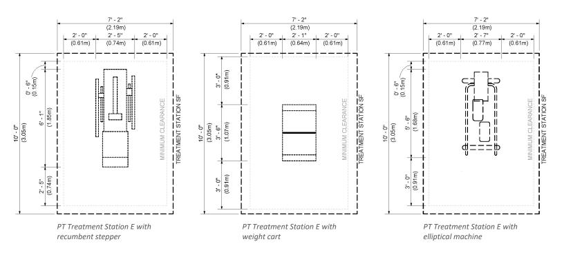
Figure 15 PT Treatment Station E with equipment options
