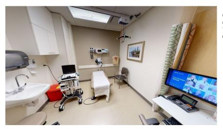
Figure 8 The PMR Svc Exam Room tables at the New Orleans VAMC are positioned to provide access on three sides.
