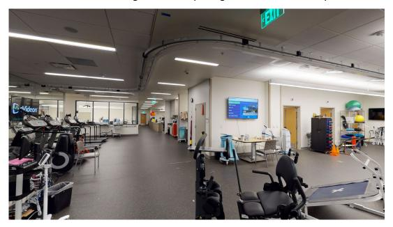
Figure 23 The OT side of the Open Treatment Area at the New Orleans VAMC includes a lift track whose path has two turns and runs over a treadmill.
