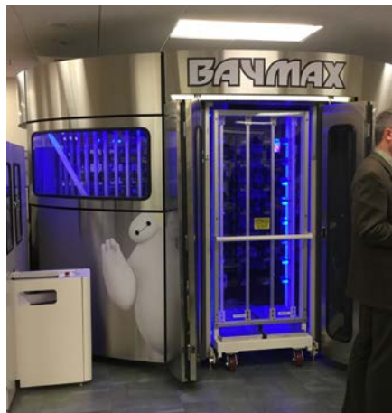
Figure 2.3 Orlando VAMC Inpatient Pharmacy Robotics
