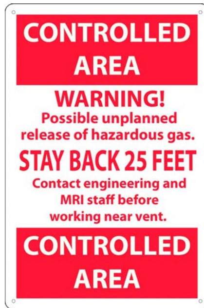
Figure 2.7.3.3-3: Example of warning signage text to be placed near quench pipe discharge or around the exclusion zone perimeter. (Image used with permission from Rutke Signs)
