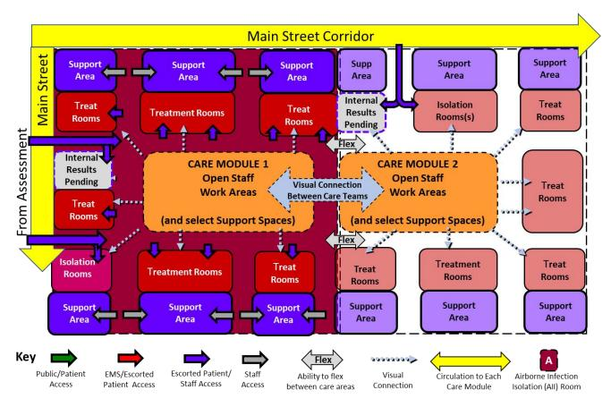
Central staff work areas shall incorporate components that will not block visibility such as: open, or glassed-in, clinical Staff Work Areas; glassed-in Consultant Provider Workstations; Equipment and cart alcoves with low-height walls; Wheelchair/Stretcher/Lift Parking alcoves; and glassed-in Medication Rooms.
