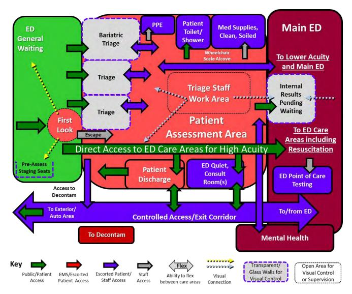
Open work/charting area should be available with visual control of triage rooms and access paths back into ED. In smaller EDs the work/charting area may be the central ED staff workstation. A wheelchair scale should be accessible. Direct access from patient assessment area to internal ED patient waiting and point of care testing should be considered.
