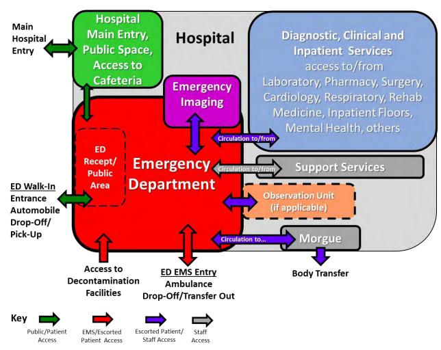
Direct access to Diagnostic Imaging is a priority and may include Emergency Imaging components within the ED. Access to Clinical/Inpatient and Support Services may include vertical transportation (elevators). Access to/from Pharmacy (for meds) and Laboratory (regarding specimen delivery) may be through a pneumatic tube system.
