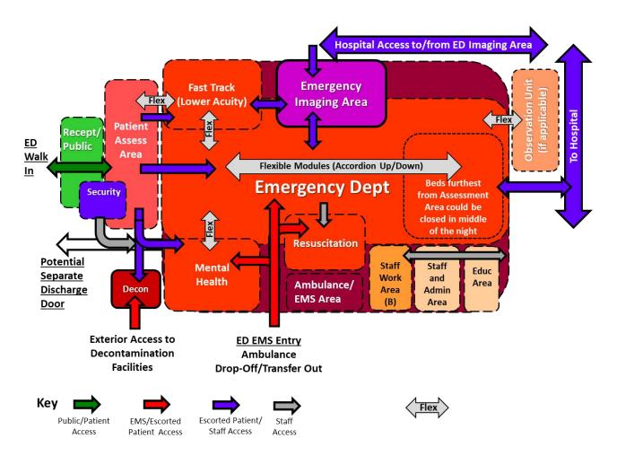
Mental health (exam / treatment or separate unit) positioned between walk-in/assessment area and EMS entry to allow immediate access for escorted patients without traveling through other care areas. EMS entry, resuscitation, and emergency imaging Area all central to main ED allowing areas to be immediately accessible to/from all parts of ED. Even in the middle of the night if beds furthest from assessment area are closed or not staffed.
