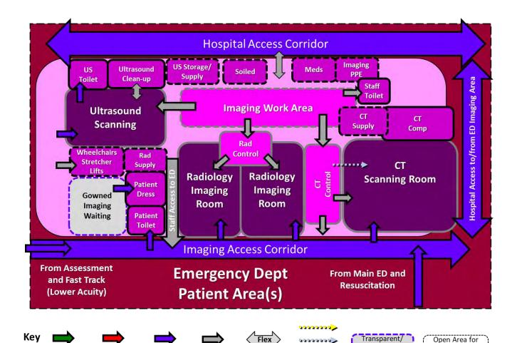
The imaging work area should have direct access to the Radiology Control Room(s), CT Control Room, Ultrasound Room, and all supply and PPE alcoves. The Ultrasound Scanning Room should have immediate access to an Ultrasound Toilet and Ultrasound Clean-up room. Consideration should be given to a pathway allowing imaging staff to leave the central Imaging Work Area to access the main ED. Orthopedic Treatment Room in the main
