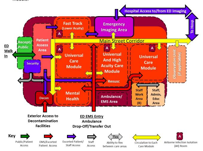
The main circulation corridor concept provides a circulation path that allows patients to come from the assessment area and circulate to any care module without traversing through other care modules. The main corridor also allows patients to come from any care module, access imaging, and return to their care module without traversing through other care modules.
