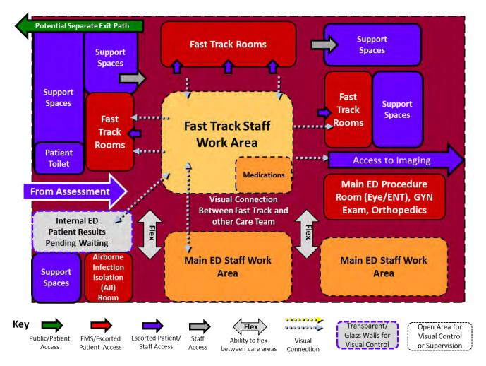
Consideration should be given to placing an Airborne Infection Isolation (AII) Room (that is in the main ED) near fast-track in case of relocation to an AII Room is deemed necessary.
