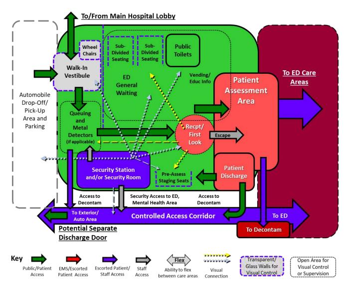
The Security Station should be positioned to allow "back door" exit to access a corridor to the main ED without traveling through the General Waiting area. There should be a clear and direct path from the entry/metal detectors to the First Look reception area (without walking through General Waiting).
