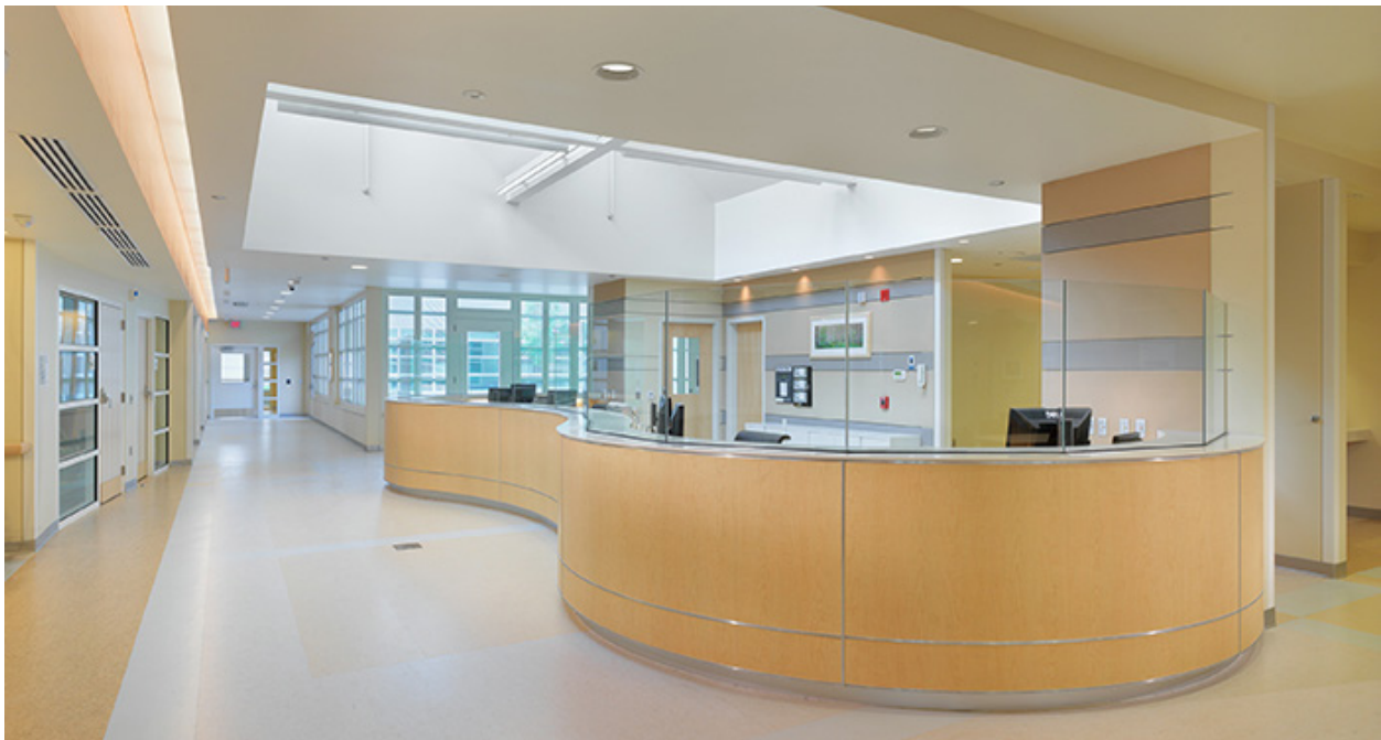
Figure 3.2 VAMC Palo Alto: The use of skylights provides additional access to daylight while also serving as way-finding landmarks. Glass partitions at the Nurse Station are used to create a secure area while also being open and inviting to patients (though open desks with no glass partitions are preferred). Off-stage Nurse Station areas (Medication Room, Team Room and Work Room) are immediately accessible behind the Nurse Station desk. These off-stage rooms provide an area of refuge for staff.
