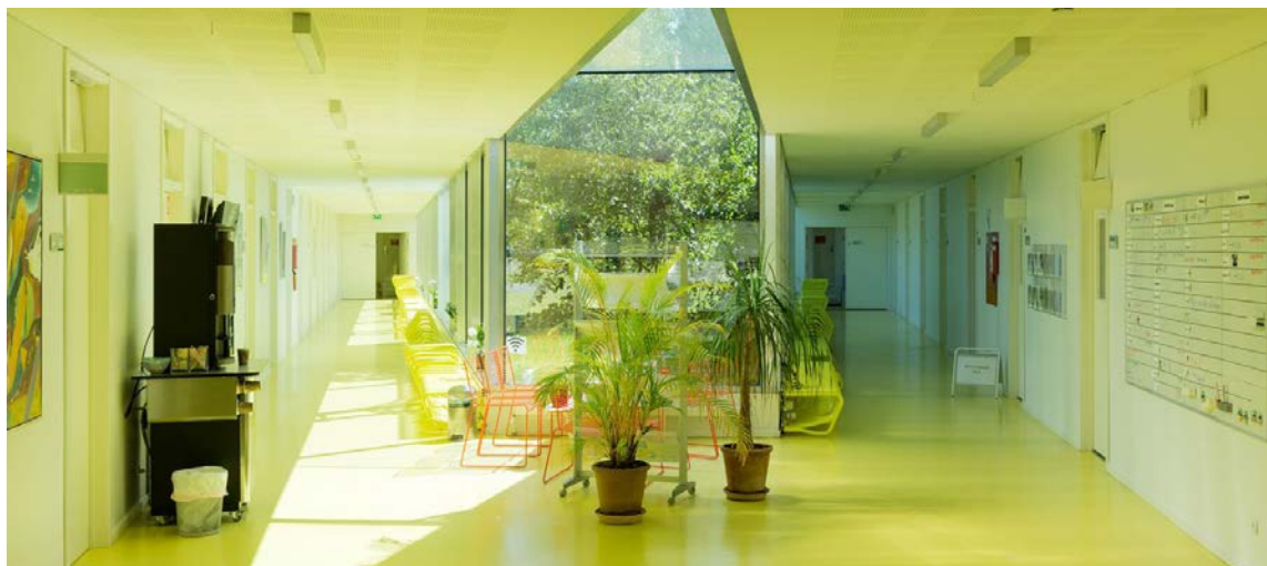
Figure 3.17 This example shows a widened circulation space to create seating arrangements, allow more space for patients to circulate through the unit to avoid altercations, access to view of nature and daylight as well as providing clear lines of sight. IKM Denmark, Helsingør, Denmark (RDS/Big)
