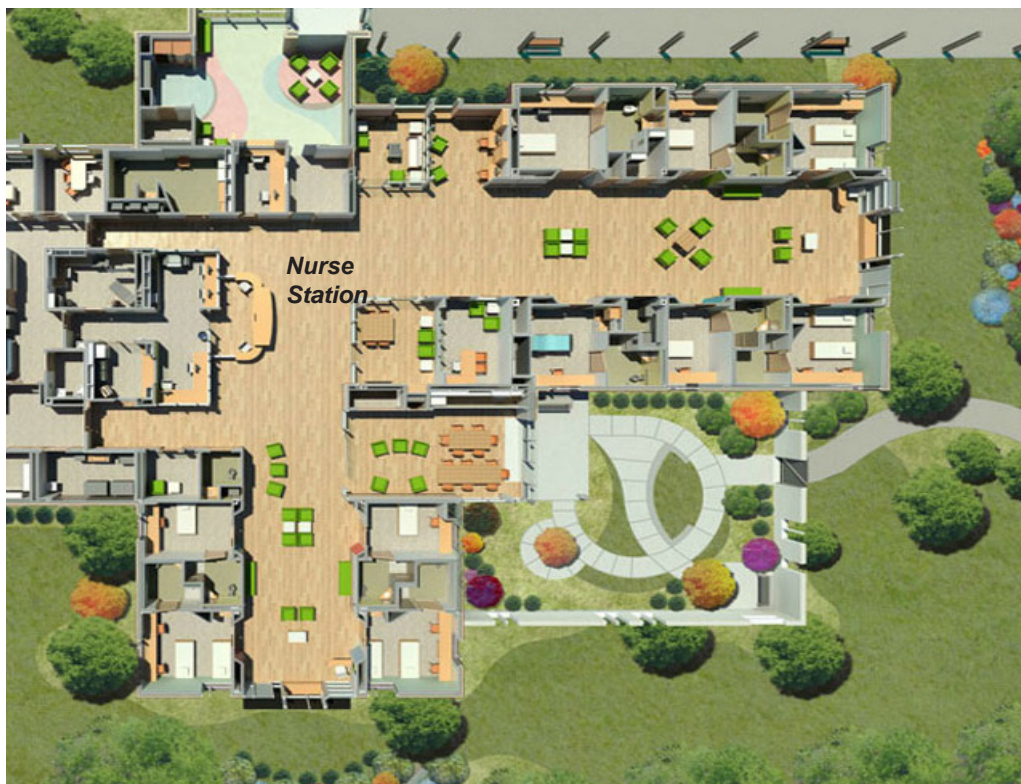
Figure 3.8 Private rooms are located closest to the Nurse Station for easy accessibility, while semi-private rooms are located at the end of the unit. Off-stage and on-stage areas are completely separated in this plan, and large windows and the end of the patient corridors provide ample access to natural daylight and views. VA Roseburg Acute Psychiatric Center, Oregon (OhPD)
