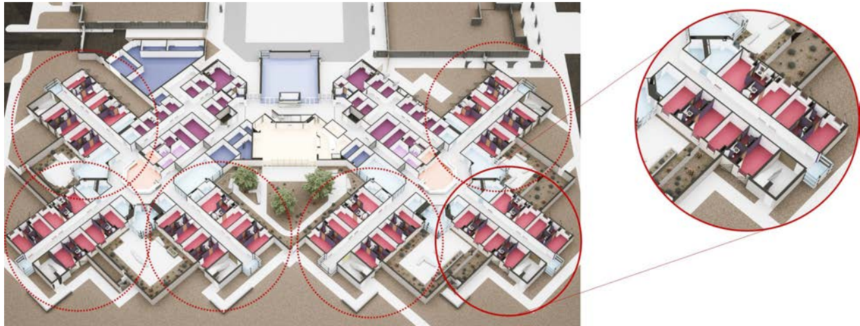
Figure 2.10 Principle #5 Example: Pod configuration creates a smaller inpatient community that improves socialization while also creating designations for specific populations. Banner Health Behavioral Hospital, Tucson, AZ, (Orcutt Wilson)
