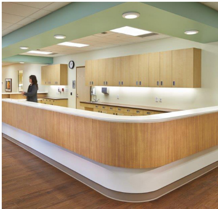
Figure 3.14 An open Nurse Station must be designed with height and depth to deter patients from jumping and/or climbing over, as demonstrated in the detail above . Everett, WA (Boulder Assoc.)
