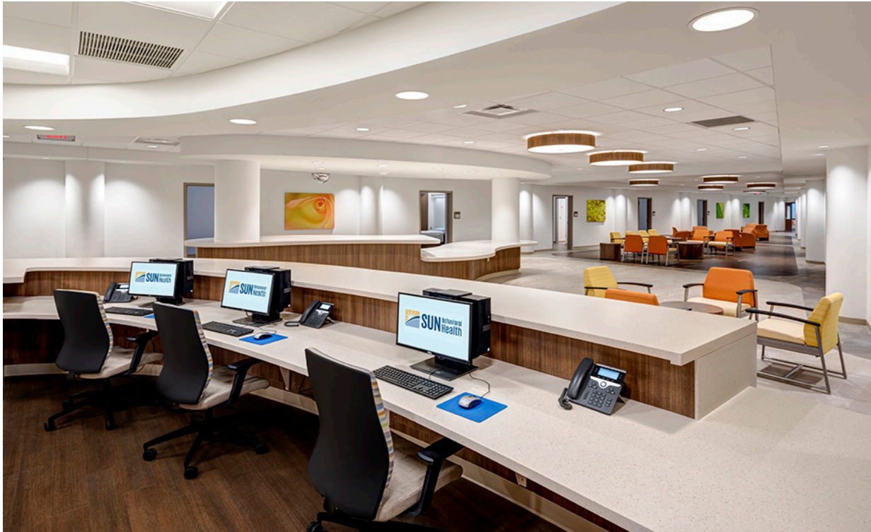
Figure 2.7 Principle #3 Example: Creating clear lines of sight from a staffed central location improves unit safety. Wide and open corridors create spaces for interaction, while also improving visibility. Sun Kentucky, Erlanger, KY, (NK Architects)
