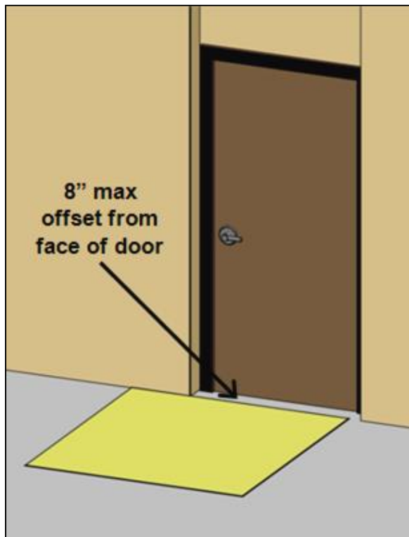
Walls and other obstructions can offset the maneuvering clearance up to 8" from the face of the door.
