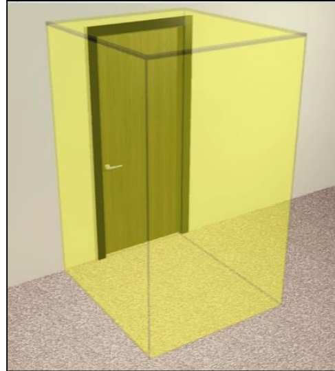
Maneuvering clearances must be free of protrusions the full height (80" min.) and changes in level (other than thresholds).
