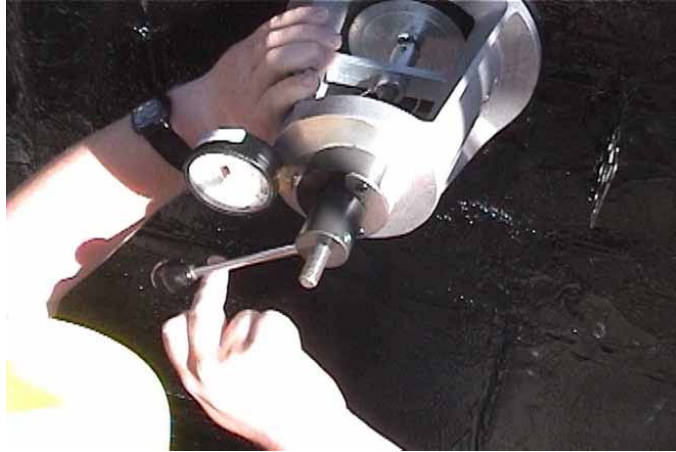
Figure 10 ASTM D 4541 adhesion pull testing
