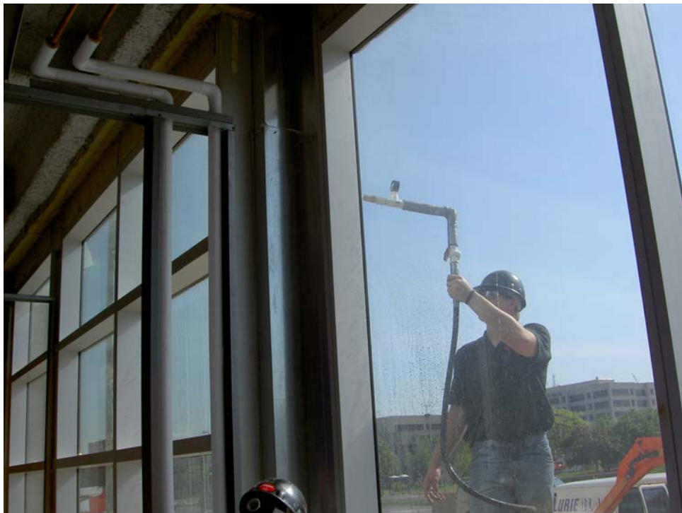
Figure 14 Hose spray testing at 15 psi, AAMA 501.2 test protocol. This is a simple test that discovers problems quickly
