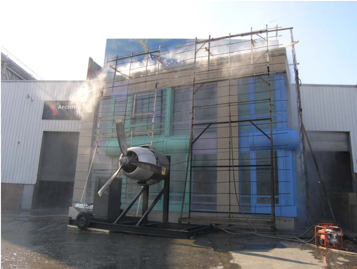
Figure 2 Dynamic Water test
