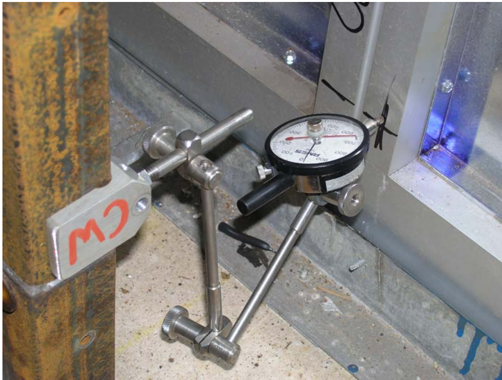
Figure 3. Strain gauges for measuring inter-story drift
