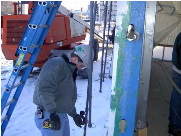
Figures 12 and 13: Field-testing of water penetration to ASTM E 1105 with spray rack.
