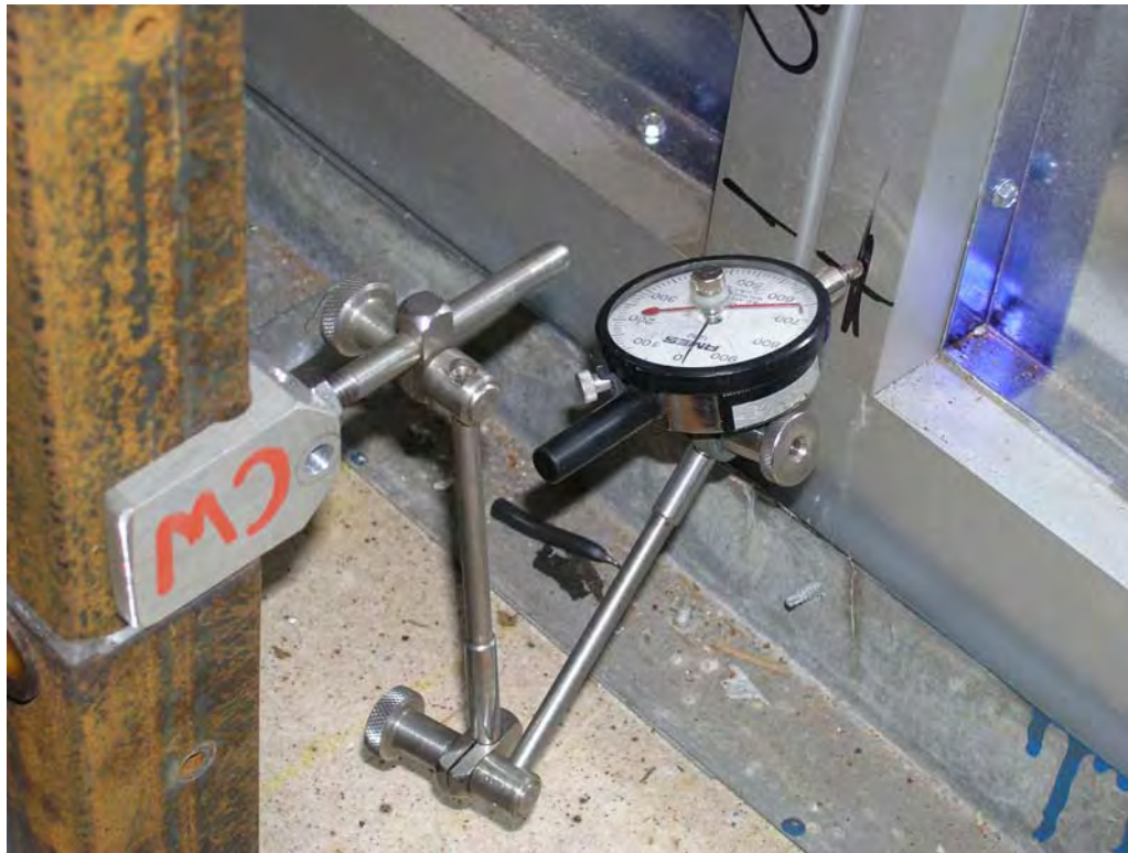
Figure 3. Strain gauges for measuring inter-story drift
