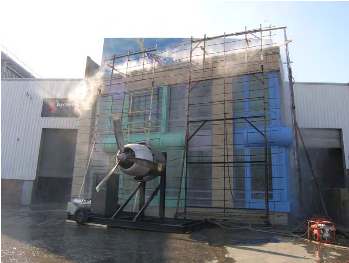
Figure 2 Dynamic Water test
