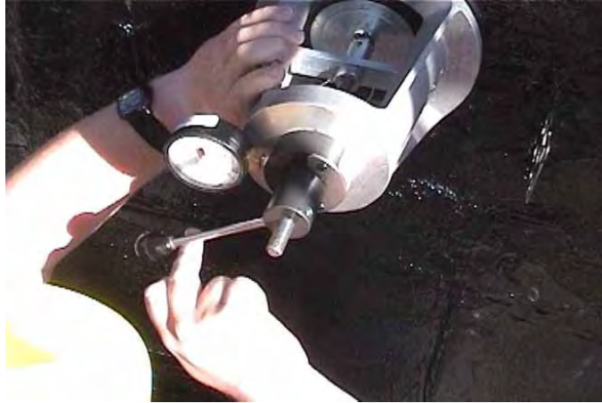
Figure 10 ASTM D 4541 adhesion pull testing
