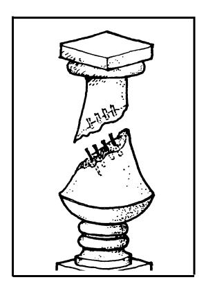
Figure 4-4. Blind Reattachment of Broken Stone.
