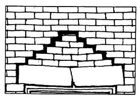
Figure 4-14. The Collapse of Masonry Lintels Indicates a Structural Fault.
