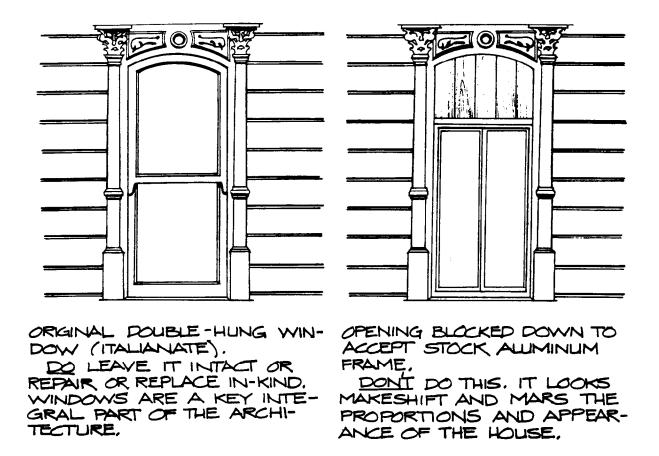
Figure 4-20. Double-Hung Window: Dos and Do nets.
