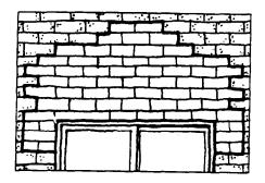
Figure 4-19. Filled-in Arch, An Inappropriate Repair.
