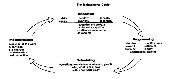
Figure 3-1. The Maintenance Cycle.
