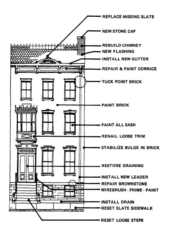
Figure 3-2. Typical Work Involved in Rehabilitating a Historic Structure.
