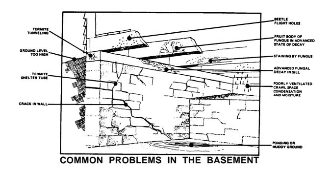
Figure 4-12. Common Problems in the Basement.
