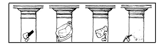
Figure 4-13. How to Apply a Poultice.
