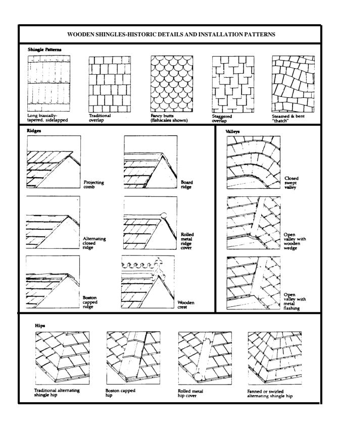
Figure 4-17. Wooden Shingles -- Historic Details and Installation Patterns.
