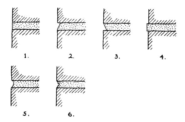
Figure 4-6. Brick Joints.
