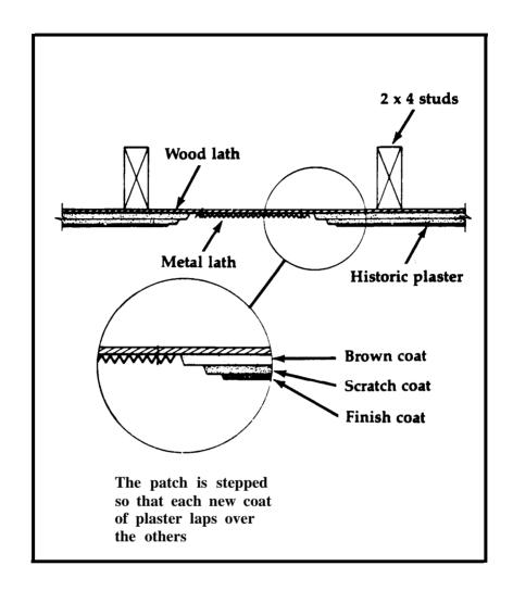
Figure 4-29. Repair of Old Plaster.
