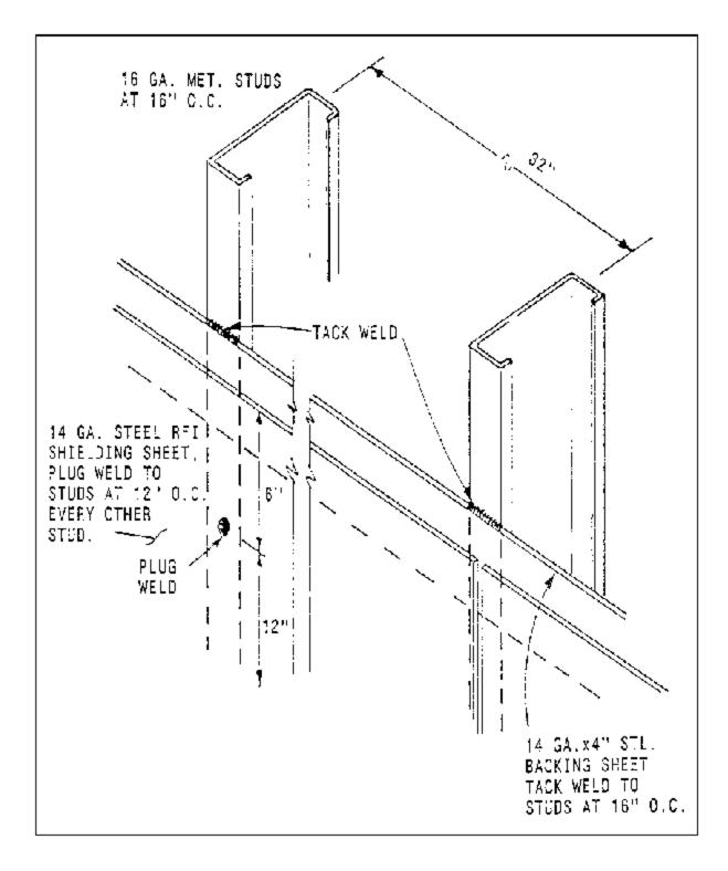
Figure 16 Welded 3F Shielding of Wall Section
