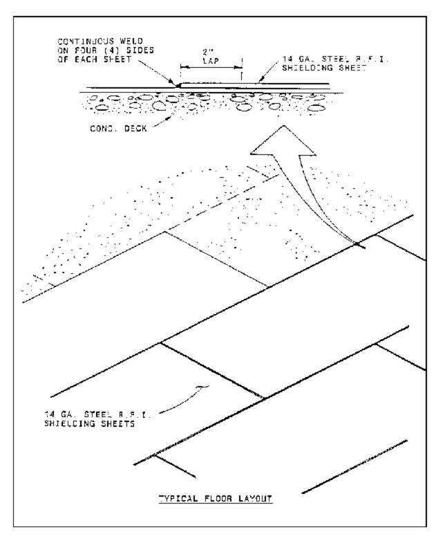
Figure 24 RF Shielding, Floor Layout
