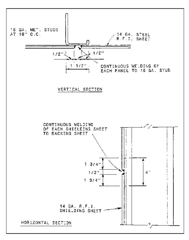
Figure 17 RF Wall Shielding, Seam Detail
