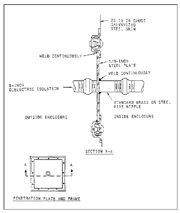
Figure 4 Single Skin Solted Enclosure Penetration Panel
