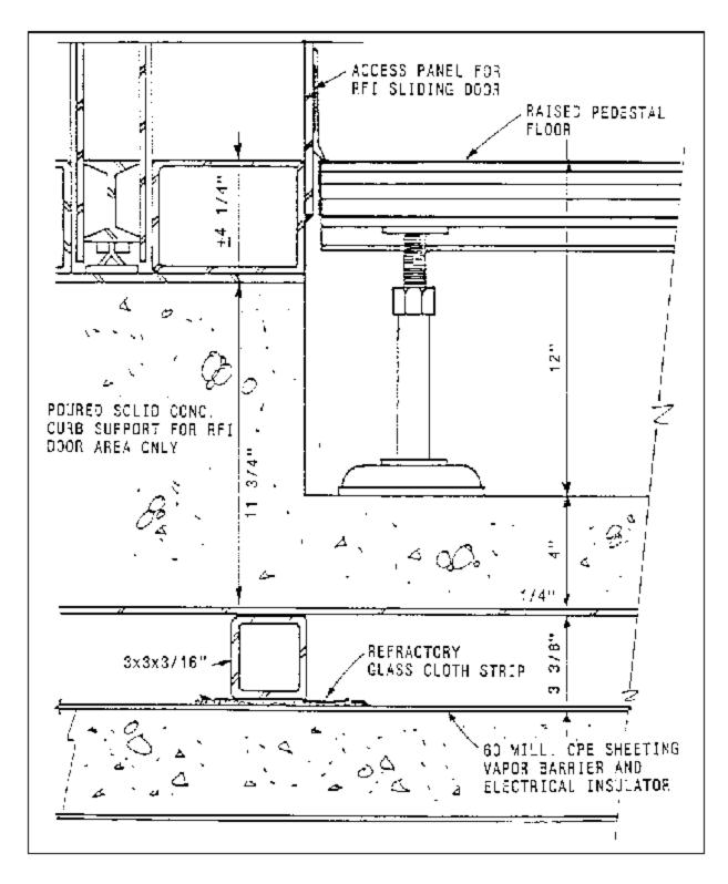
Figure 20 RF Shielding, Sliding Door Frame Section
