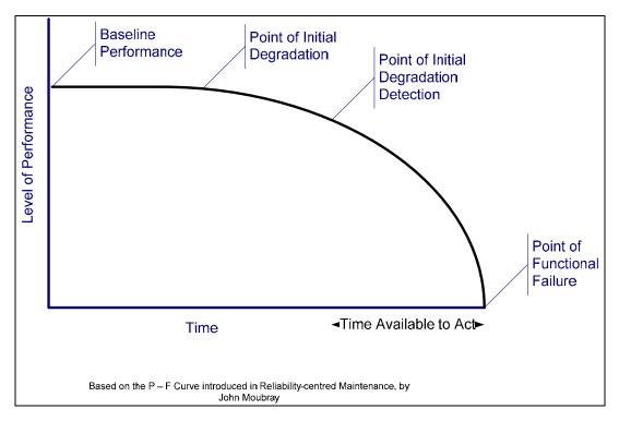
Figure 4-2. P-F Curve (Modified)
