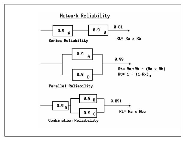
Figure 5-4. Determining Network Reliability
