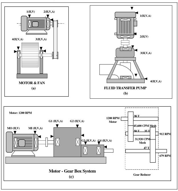
Figure E-6. Vibration Measurement Locations
