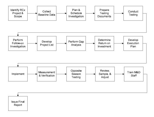
Figure 13-1. The Retrocommissioning Process
