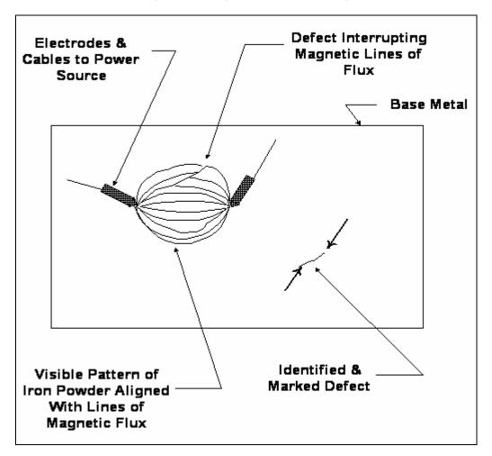
Figure 6-6. Magnetic Particle Testing
