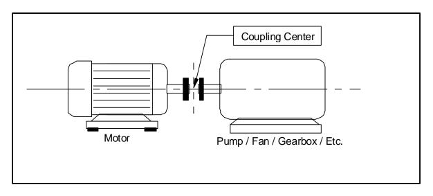
Figure G-1. Coupled Shafts Alignment
