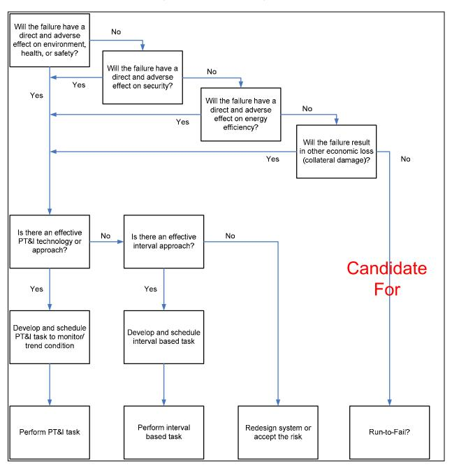
Figure 3-2. NASA RCM Logic Tree
