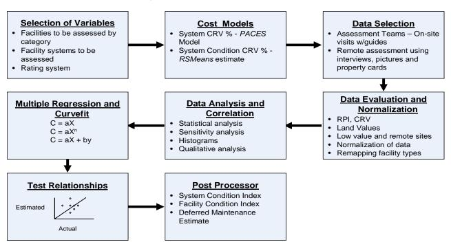
Figure 5-6. Generic Parametric Model
