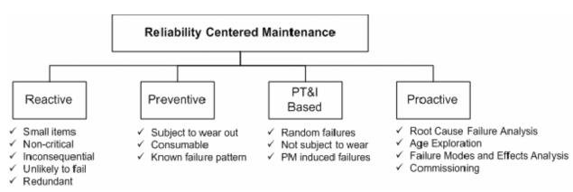
Figure 3-1. Components of an RCM Program
