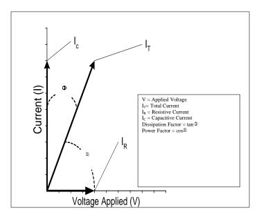
Figure 6-3. Power Factor Current/Voltage Relationship
