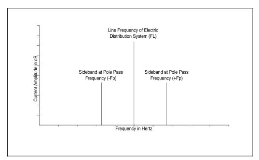
Figure B-17: Simplified Motor Current Signature
