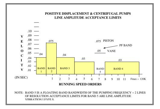
Figure 2-13: Positive Displacement and Centrifugal Pump Vibration Envelope Overall Per Band
