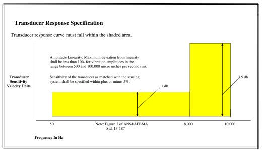
Figure 2-1: Transducer Response
