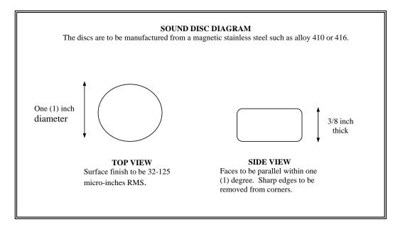
Figure B-5: Sound Disc Diagram
