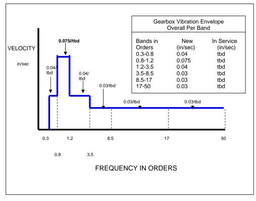
Figure 2-8: Gearbox Vibration Envelope Overall Per Band
