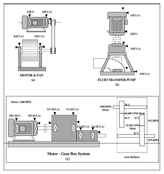
Figure B-4: Typical Vibration Measurement Locations
