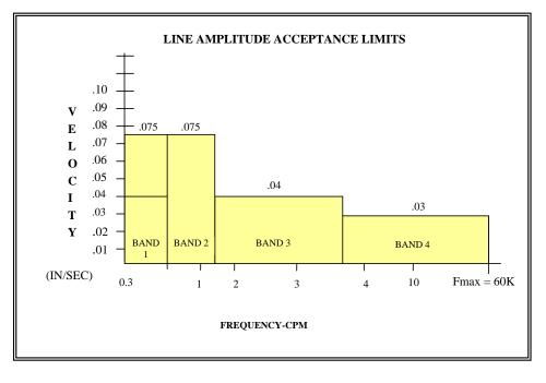
Figure 2-2: Belt Driven Blower Vibration Envelope Overall Per Band
