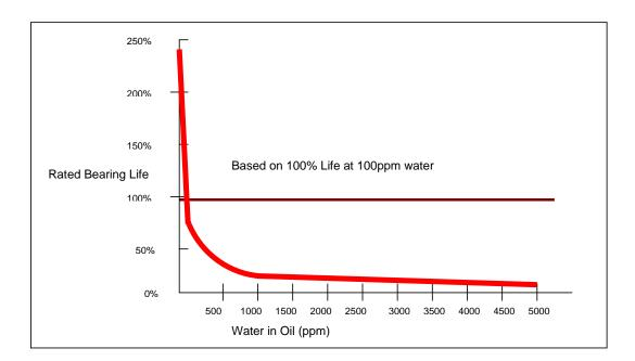
Figure B-15: Bearing Life Reduction from Water in Oil<sup>13</sup>
