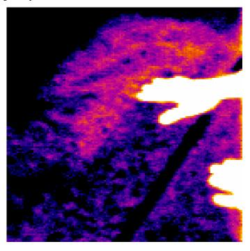
Figure 2-14: Infrared Image of Moisture Under Roof<sup>8</sup>
