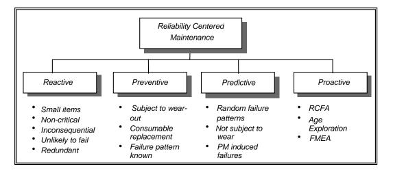
Figure A-1: Components of an RCM Program
