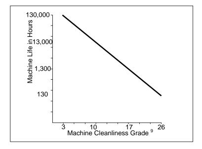
Figure B-14: The Effect of Hydraulic System Contamination<sup>12</sup>
