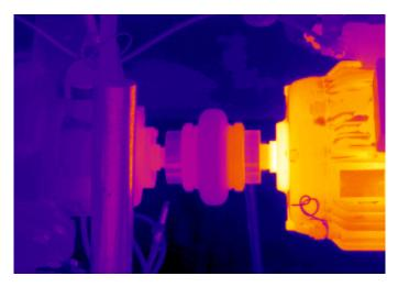
Figure B-10: Infrared Image of Motor/coupling<sup>11</sup>
