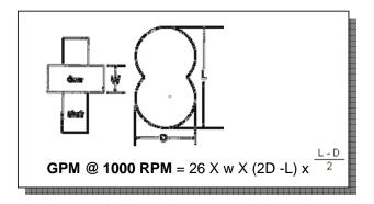
Figure 2-12: Figuring Gear Pump G.P.M.
