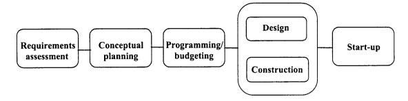
FIGURE 2-2 General facility acquisition process.
