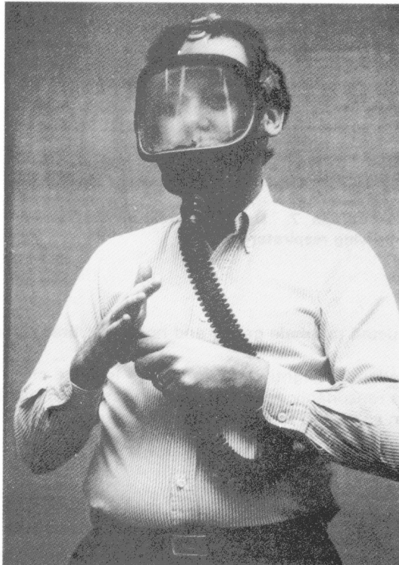
Photograph 6. Negative pressure test on SAR or SCBA.
