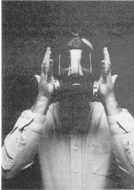
Photograph 7. Negative pressure test on air-purifying respirator.
