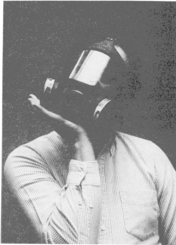
Photograph 8. Positive pressure test; blocking exhalation valve.
