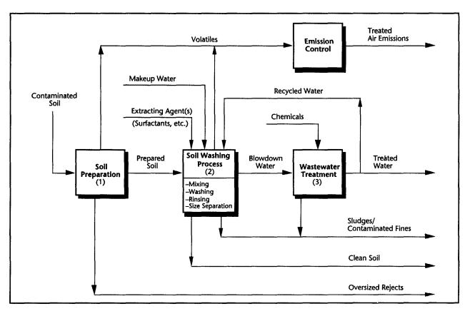
Figure 2-1. Schematic diagram of the major elements of the aqueous soil washing process.
