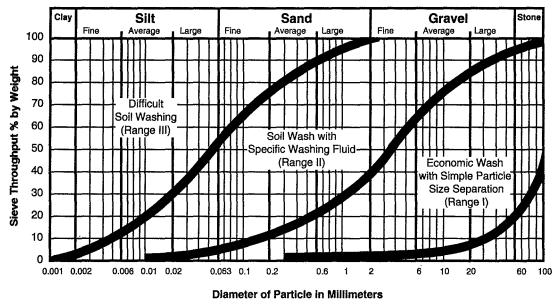
FIGURE 4-1. Soil washing applicable particle size range.
