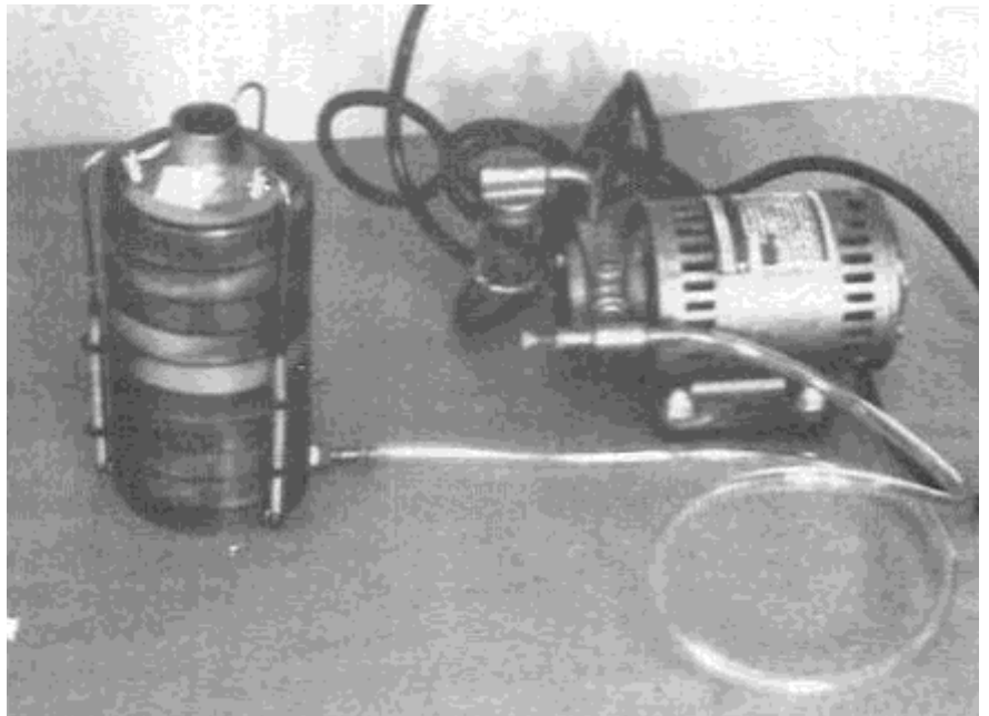
A viable impactor. Used to sample for biologicals. Training is required in order to analyze the results.
