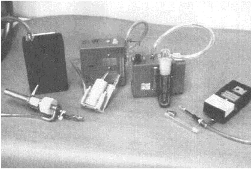
A vacuum pump with attachments for sampling with a filter, a sorbent tube, and an impinger. Use in a non-industrial setting may require a larger volume of air. Consult with qualified industrial hygienists and chemists if adapting sampling methods.
