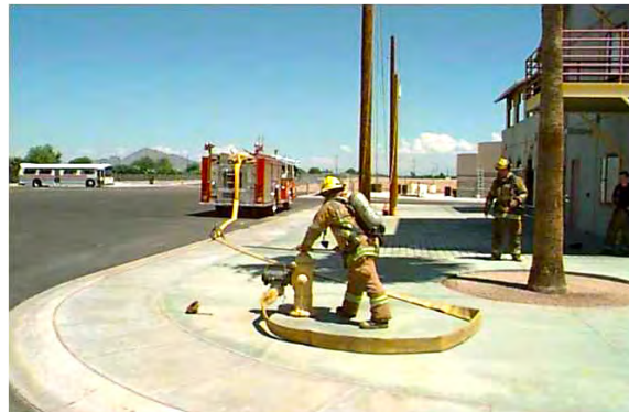
Figure 4.11. The same pumper completing the straight lay towards the fire scene, and a firefighter preparing to operate the hydrant.
