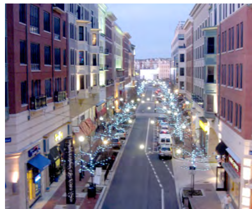
Figure 3.7. Lights strung across this street preclude the use of aerial ladders and limit the use of portable ladders.
