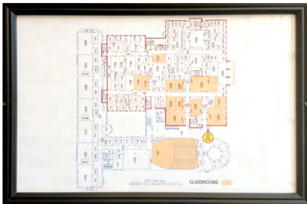
Figure 6.8. A building diagram with the building features oriented properly but the text turned 90 degrees from the viewing angle.
