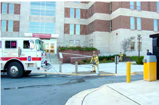
Figure 2.7. During initial operation at this structure, the first arriving engine crew is already using a fire lane, a fire hydrant, the fire department connection, and the key box. Interior operation will soon involve the alarm system, stairs, standpipe system, and other building features.
