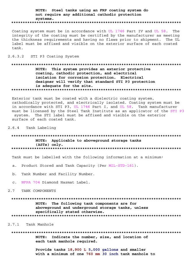
allow for internal tank access. Provide tanks larger than 18,900 L 5,000 gallons with a minimum of two 915 mm (36 inch) tank manholes (one manhole for access). Diesel and bio-diesel tanks at military service stations are to be provided with a 813 mm (32 inch) access manhole. Piping will not penetrate through access manholes.
