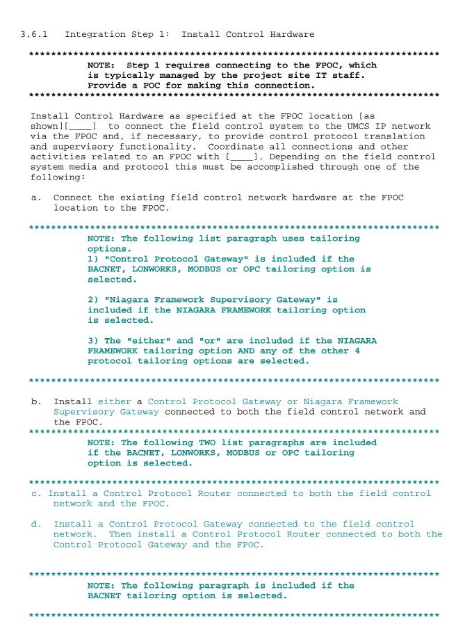
In addition, for integration of field control systems via ASHRAE 135, also install a BACnet Supervisory Controller as needed to implement scheduling, alarming and trending in the field control system. The BACnet supervisory controller may be the same device as the control protocol gateway or router.
