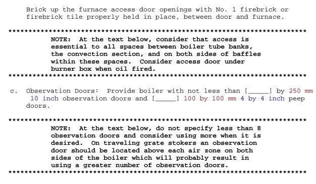
d. Door and Opening Frames: Frames and front plates for openings for doors, soot blowers, overfire air openings, and other such items, in the pressure parts shall be completely gastight and airtight. Doors shall close against planed seats or the equivalent and shall be provided with heavy latches. Anchor door frames securely. There shall be no air leaks between door frames and setting.
