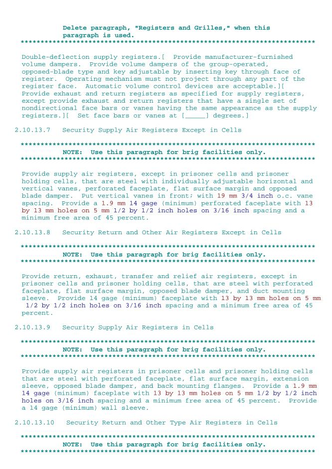
Provide steel return, exhaust, transfer and relief air registers in prisoner cells and prisoner holding cells with perforated faceplate, flat surface margin, wall sleeve, opposed blade damper, and back mounting flanges. Provide 1.9 mm 14 gage (minimum) faceplate with 13 by 13 mm holes on 5 mm 1/2 by 1/2 inch holes on 3/16 inch spacing and a minimum free area of 45 percent. Provide a 14 gage (minimum)wall sleeve.
