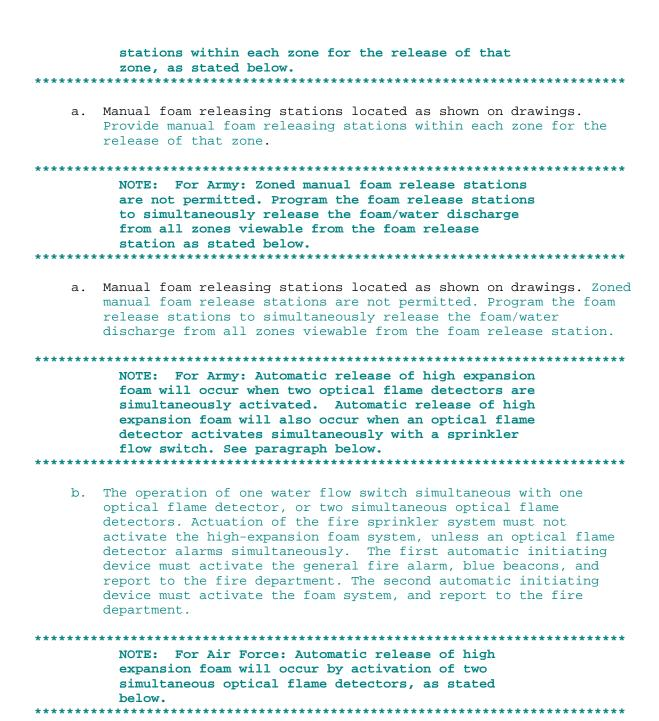
b. The simultaneous operation of two optical flame detector in the hangar bay is required to automatically release the high-expansion foam. Actuation of the fire sprinkler system must not activate the high-expansion foam system. The first optical flame detector must activate the general fire alarm, the blue beacons, and report to the fire department. The second optical flame detector must activate the foam system, and report to the fire department.
