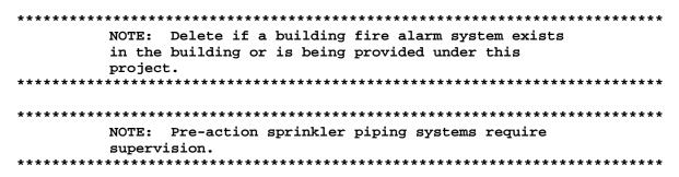
Provide local [ 100 mm 4 inch] electric alarm [bell] [horn] [\_\_\_\_] to indicate trouble [or failure of the [detection system] [ or ] [pre-action sprinkler piping system]]. Also connect trouble alarm into the building fire alarm control panel to indicate "trouble" on a separate zone labeled "Foam System Trouble".
