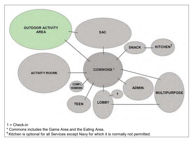
FIGURE 2-3. FUNCTIONAL RELATIONSHIP BUBBLE DIAGRAM
