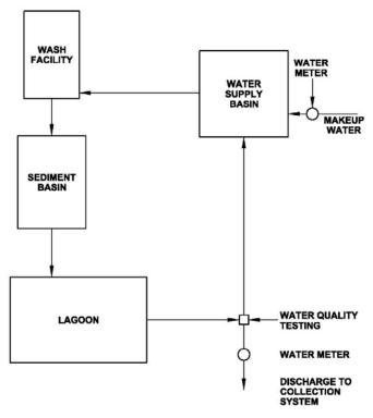
Figure 6-19 General Flow Schematic of a Lagoon System
