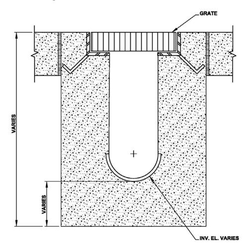
Figure 4-7 Cross Section of a Trench Drain
