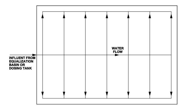
Figure 6-13 Distribution System Using Grid Arrangement
