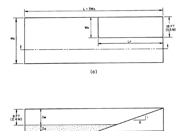
c. Sediment Volume. The designer estimates that the installation has average-to-heavy soiling conditions. By applying Stokes Law, using  $Q_{over}$  with the basin size previously calculated, and checking the soil particle size
