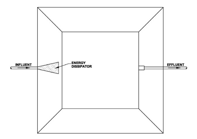
Figure 6-23 Water Supply Basin, Cross Section
