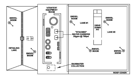
Figure 8-5 Dual Lane, Net Zero Wash Lane with Heavy Solids and Detailing Lanes
