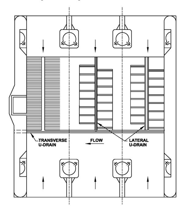
Figure 5- 10 Configuration of U-Drains in the Bath
