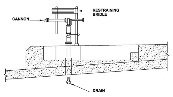
Figure 5-5 Example Cross Section of a Cannon Island
