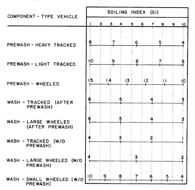
Figure 3-4 Vehicle Processing Rates (Vehicles per Hour)
