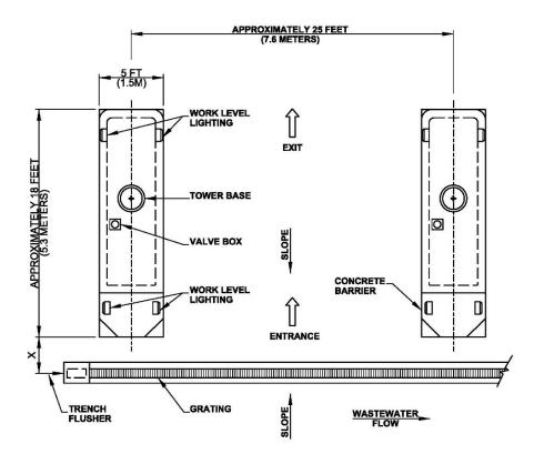
Figure 4-2 Wash Island Plan Showing Spacing
