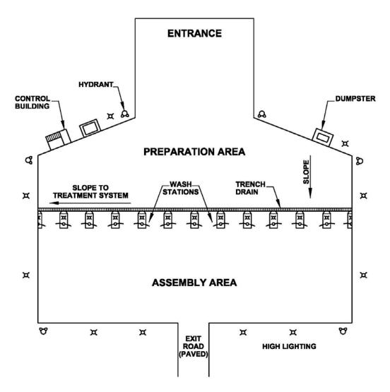
Figure 2-1 Standard Central Vehicle Wash Facility Plan
