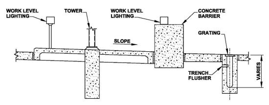
Figure 4-5 Longitudinal Section of an Island
