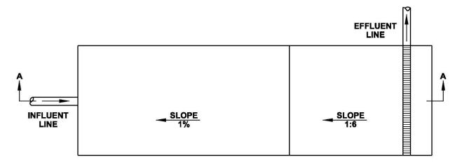
Figure 6-2 Single Cell Sediment Basin, Cross Section
