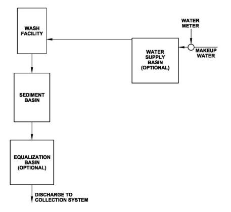
Figure 6-21 General Flow Schematic of a Total Discharge System
