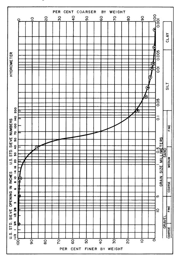
Figure 3-2 Noncohesive Soil Gradation Curve
