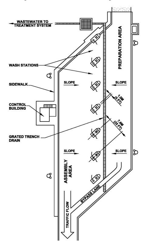
Figure 4-1 Skewed Wash Station Arrangement
