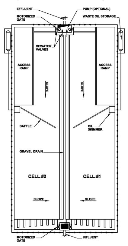
Figure 6-8 Sedimentation Basin Drain System
