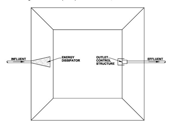
Figure 6-11 Example Equalization Basin, Plan View
