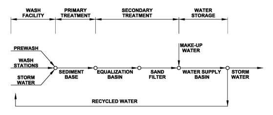
Figure 6-9 Components of an Intermittent Sand Filter System
