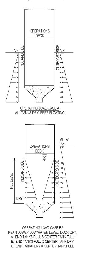
Figure 9-5 Example Load Cases for Caisson – 1 of 2
