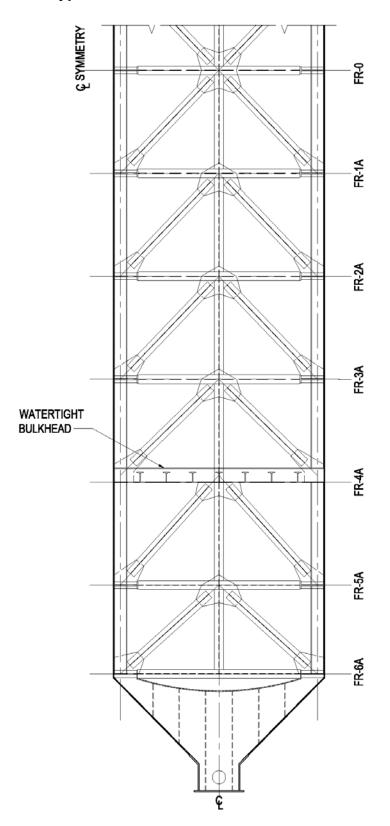
Figure 9-4 Typical Horizontal Girder for Welded Caisson
