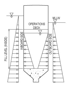
OPERATING LOAD CASE C MEAN LOWER LOW WATER LEVEL OUTSIDE, DOCK SUPER FLOODED, END TANKS FULL & CENTER TANK FULL
