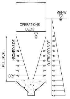
OPERATING LOAD CASE B1 MEAN HIGHER HIGH WATER LEVEL OUTSIDE, DOCK DRY, A. END TANKS FULL & CENTER TANK FULL B. END TANKS FULL & CENTER TANK DRY C. END TANKS DRY & CENTER TANK FULL
