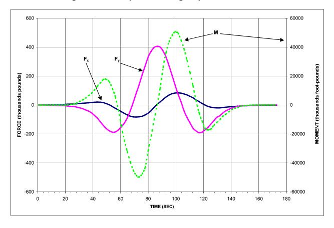
Figure 9-2 Example of Passing Ship Predictions
