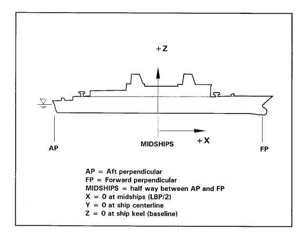
Figure 3-4 Local Mooring Coordinate System for a Ship
