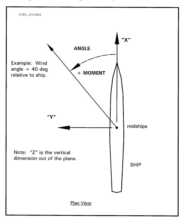
Figure 3-3 Local Mooring Coordinate System for a Ship
