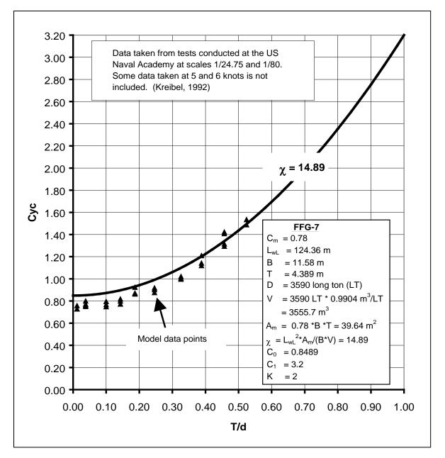
Figure 4-11 Example of Transverse Current Drag Coefficients
