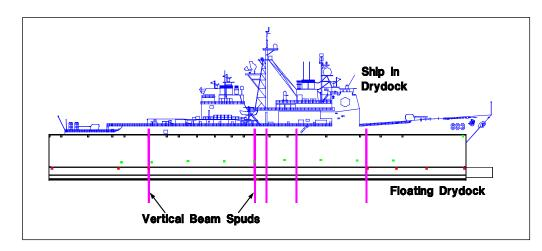
(spuds are secured to a pier, which is not shown, and the floating dry dock rides up and down on the spuds; profile view is shown)
