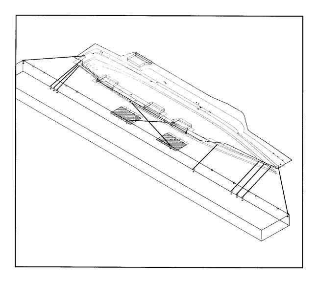
Figure 8-12 Aircraft Carrier Mooring Concept (perspective view)
