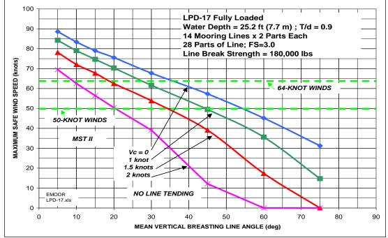
Six degree of freedom quasi-static analyses using the program ANSYS AQWA are performed on various LPD 17 mooring configurations to determine safe mooring limits as follows:
