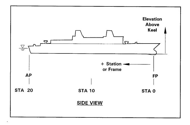
Figure 3-2 Ship Design and Hydrostatic Coordinates
