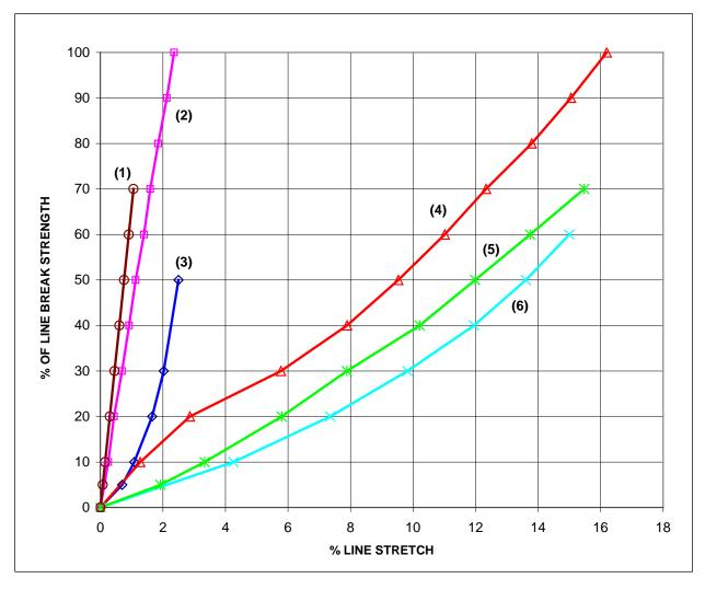
Figure 6-2 Synthetic Line Stretch
