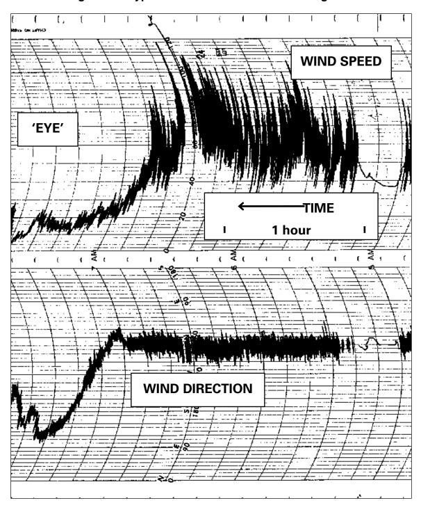
Figure 3-6 Typhoon Omar Wind Chart Recording
