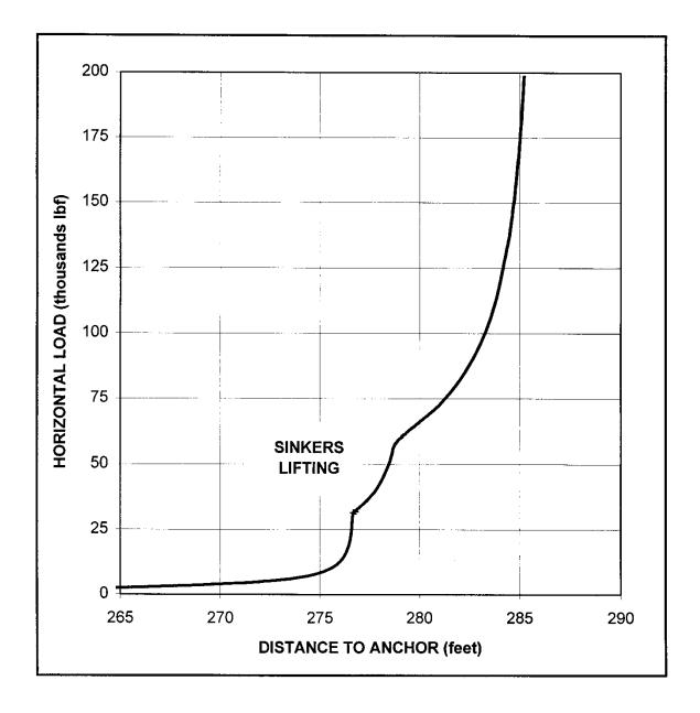
Figure 6-5 Load/Deflection Curve for the Example Mooring Leg
