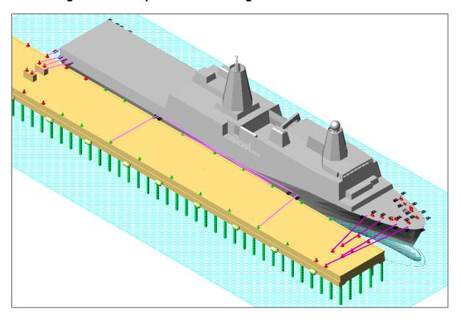
Figure 8-25 Sample LPD-17 Mooring at a Double-Deck Pier
