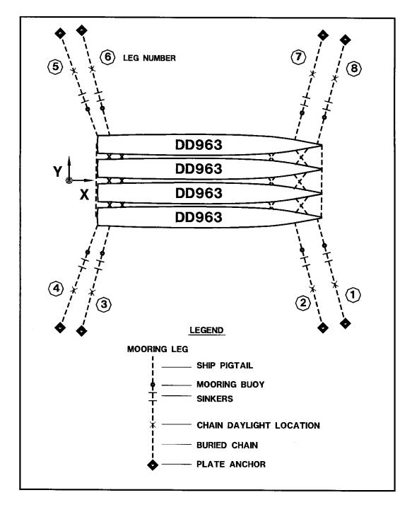
Figure 8-14 Spread Mooring Arrangement for a Nest of Four Destroyers
