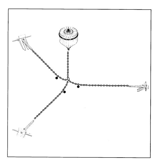
Figure 2-7 Single Point Mooring with Drag Anchors
