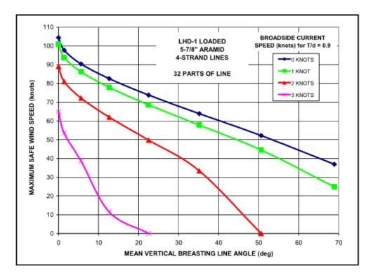
Figure 8-18 LHD 1 Safe Mooring Limits from 32 Part Line
