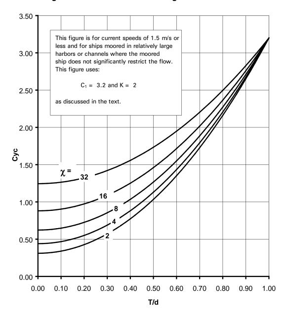
Figure 4-9 Broadside Current Drag Coefficient
