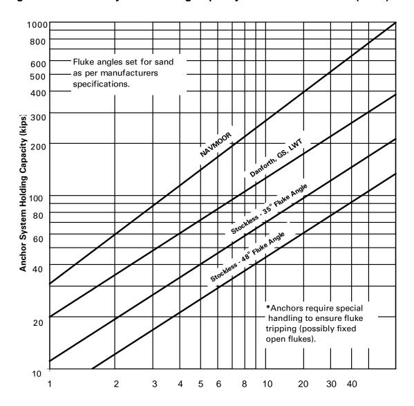
Figure 5-5 Anchor System Holding Capacity in Cohesionless Soil (Sand)
