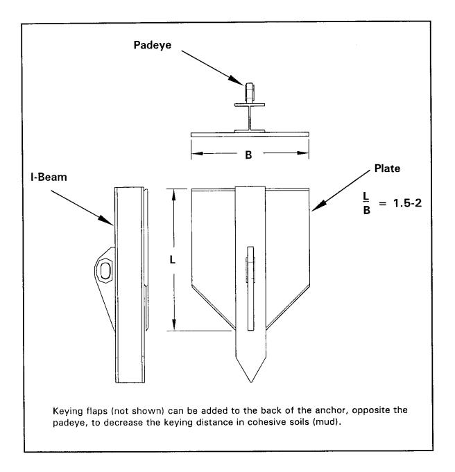
Figure 5-3 Driven-Plate Anchor
