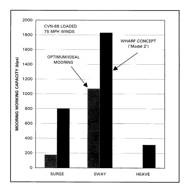
Figure 8-10 Component Analysis of Mooring Working Capacity
