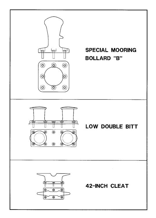
Figure 6-3 Pier and Wharf Mooring Fittings Shown in Profile and Plan Views
