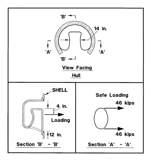
Figure 7-2 Recessed Shell Bitt (minimum strength requirements)
