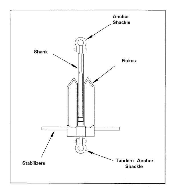
Figure 5-2 Example of a Drag-Embedment Anchor (NAVMOOR Anchor)
