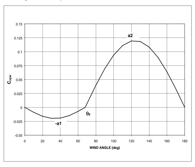
Figure 4-7 Example Normalized Yaw Wind Moment Coefficient
