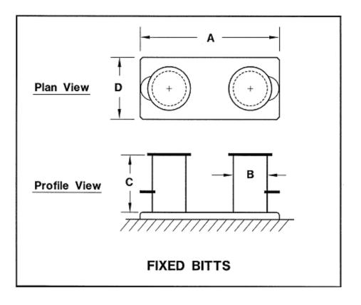
Figure 7-1 Ship's Fixed Double Bitts
