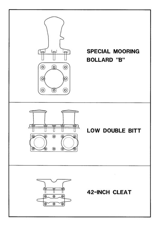
Figure 2-3 Typical Profiles of Mooring Hardware
