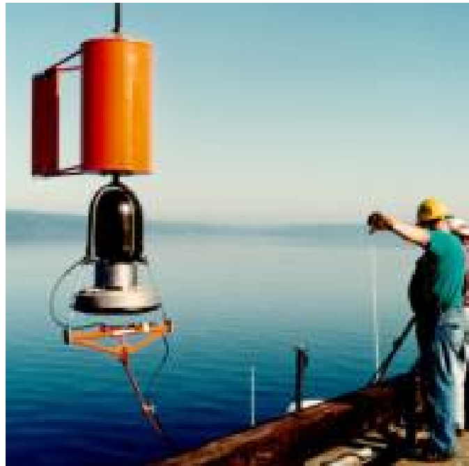
Figure 5-5 Sound Transducer Being Lowered into the Water
