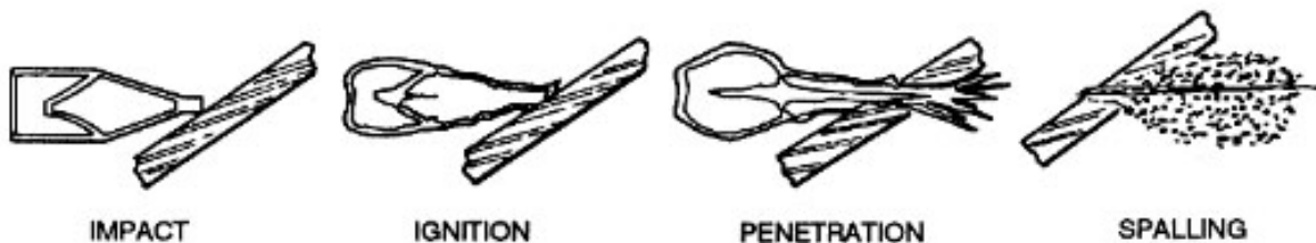
Figure 2-2. Shaped Charge Penetration
