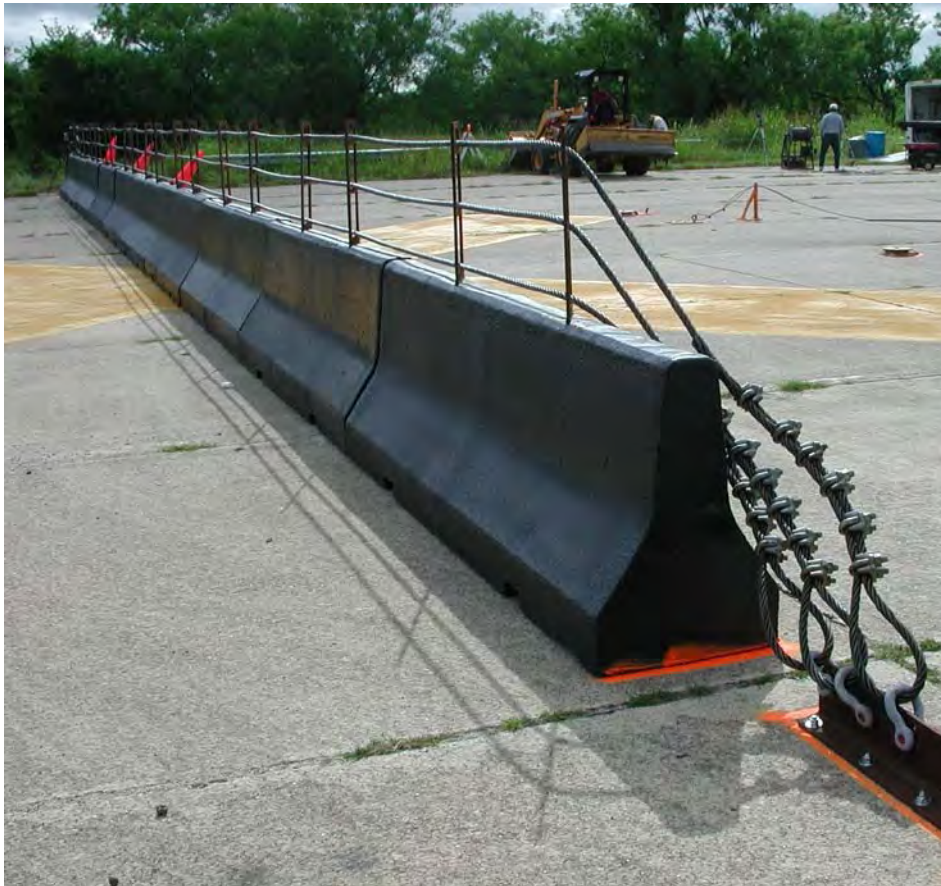
Figure E-4 Polymer-Coated, Lightweight Concrete Barrier System
