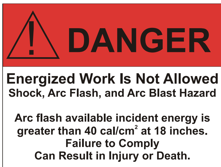
Figure 1-11 Arc Flash Danger Label for Locations Identified to Be Greater Than 40 cal/cm 2
