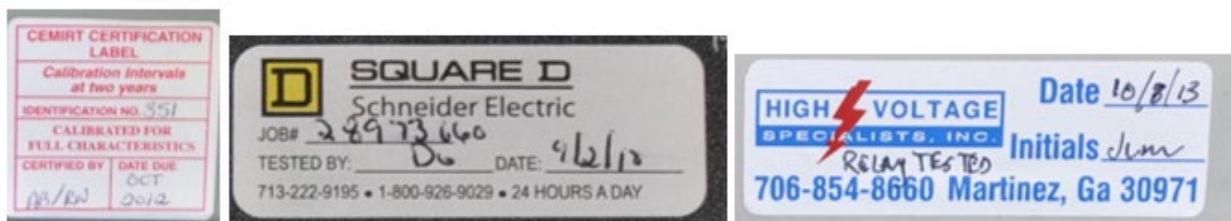
Figure 1-5 Typical Calibration or Maintenance Stickers
