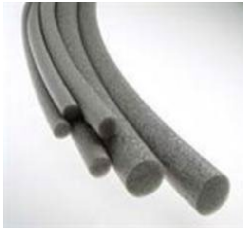
Figure 9-10 Examples of Backer Rod Materials
