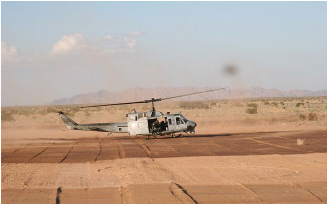
Figure 5-7 UH-1 Rotary-Wing Aircraft Operating on Treated Helipad
