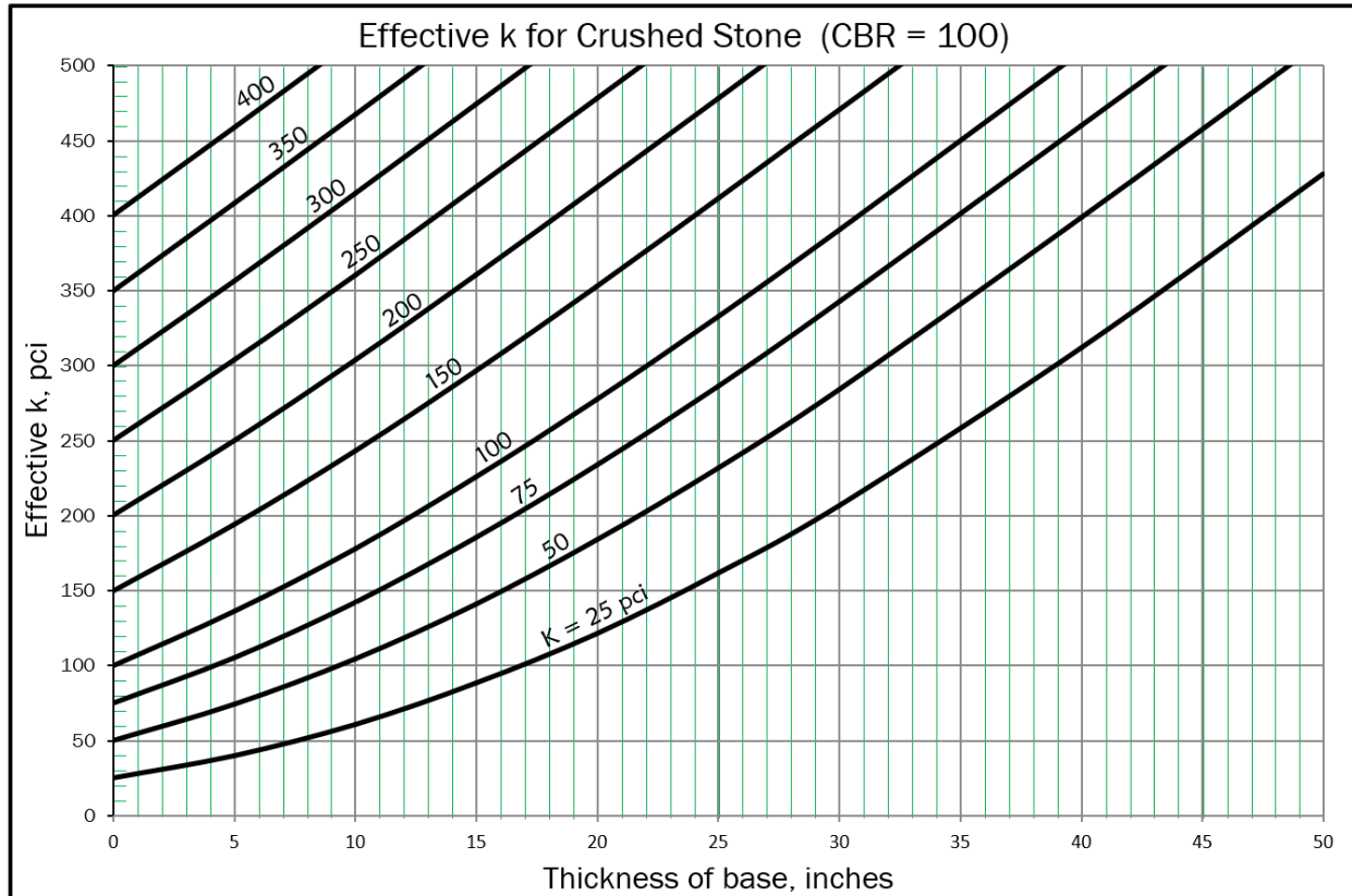
Figure 7-10 Effective k Crushed Stone Base Course Determination
