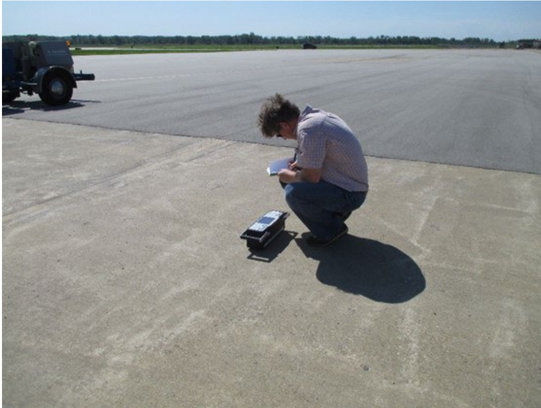
Figure 3-8 MIRA Ultrasonic Tomography
