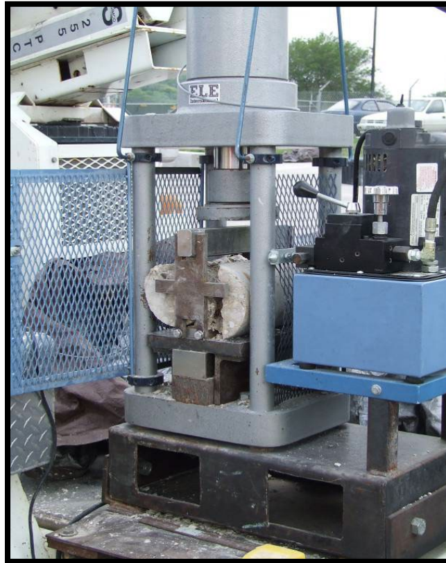
Figure A-1 Portable Split Tensile Tester
