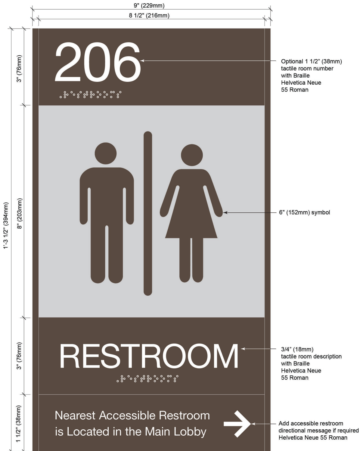
1\1 Figure 4-5 Non-Accessible Restroom Identification Signs. /1/
