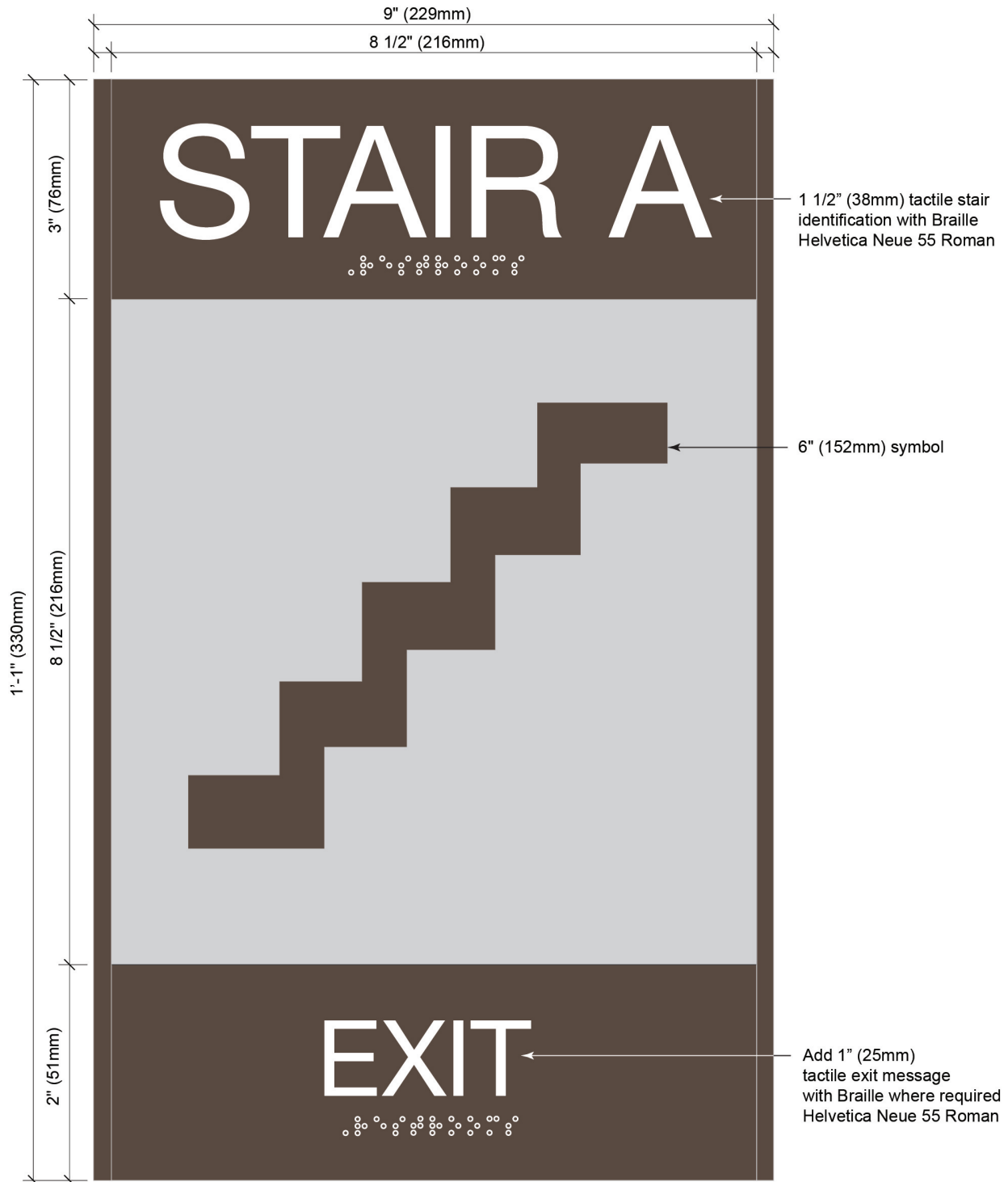
1\1 Figure 4-6 Stair Identification Signs. /1/
