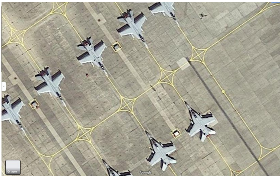
Figure 2-3 Example of Apron Layout with POU Equipment
