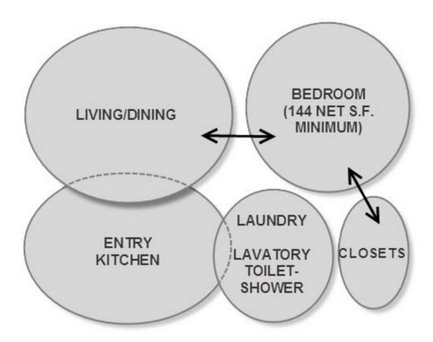
Figure B-3 Navy 2+0 Unit Bubble Diagram
