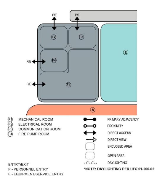
Figure 3-27 Module F Adjacency Diagram
