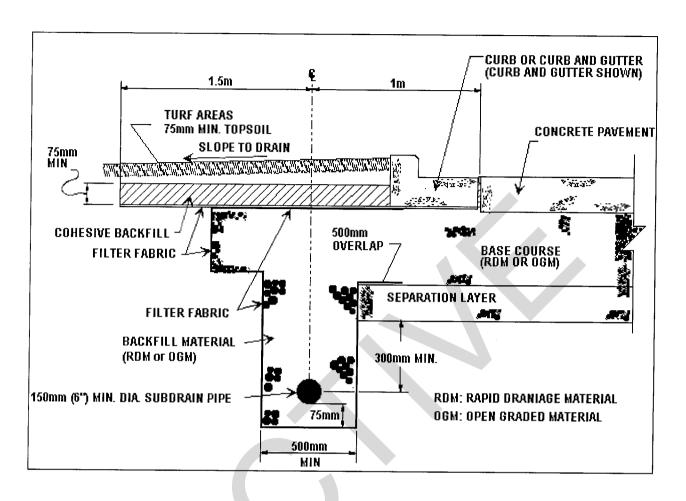
Figure 5-3. Typical Edge Subdrain Detail for Concrete Pavements.
