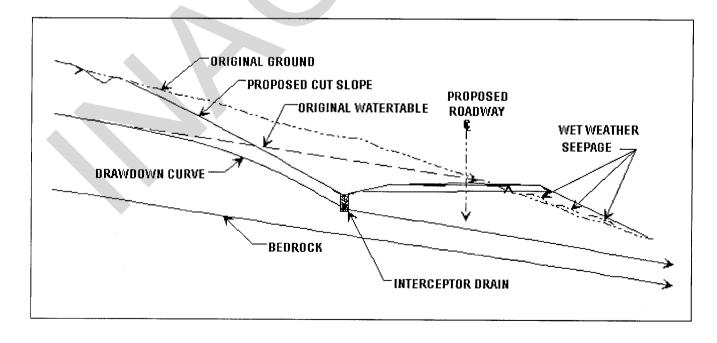
Figure 1-2. Collector Drain Used to Intercept Seepage and Lower the Groundwater Table.
