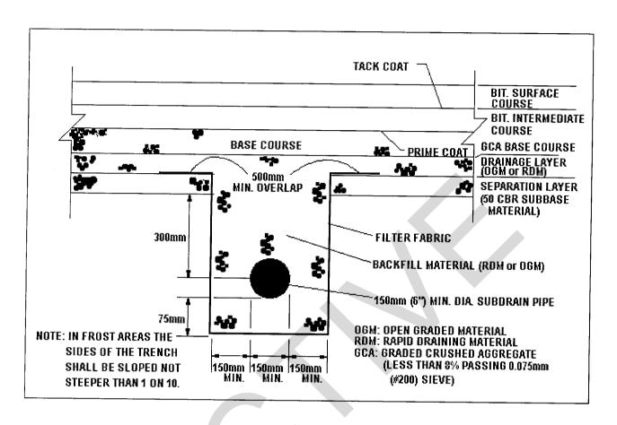
Figure 5-4. Typical Flexible Pavement Interior Subdrain Detail.
