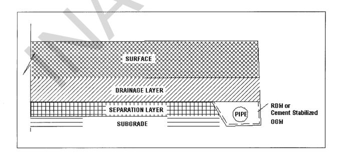
Figure 3-2. Drainage Layer Placed Directly Below Surface Layer.
