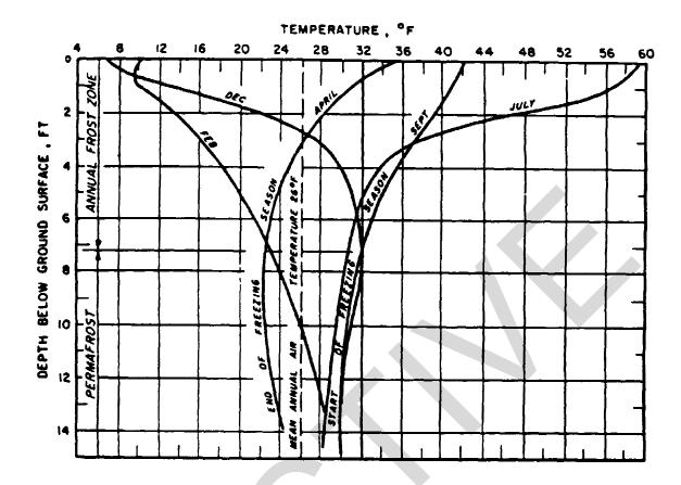
Figure 4-1. Typical ground temperatures, Fairbanks, Alaska.
